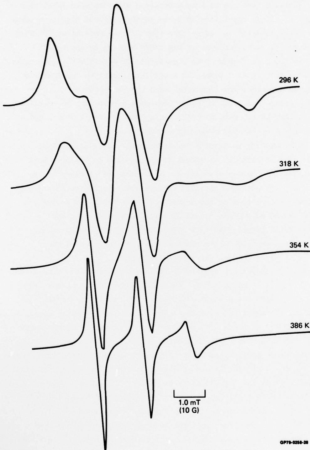
Figure 55 Spectra observed at 296 K, 318 K, 354 K, and 386 K from spin label II in nonreverted polyurethane.
