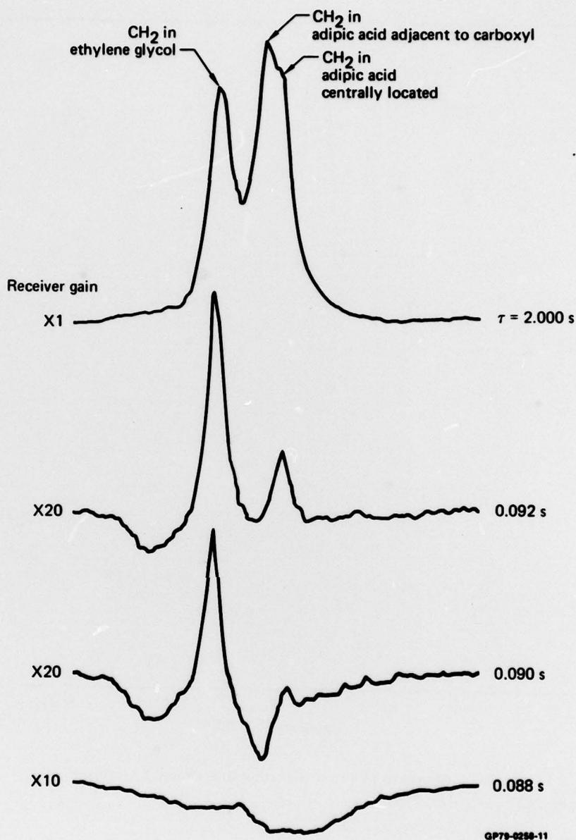
Figure 59 Partially spin-lattice relaxed spectra of polyurethane after 30 h exposure to 363 K 100% relative humidity.  $\tau$  is the time between the spin-inverting pulse and the sampling of the spectra.
