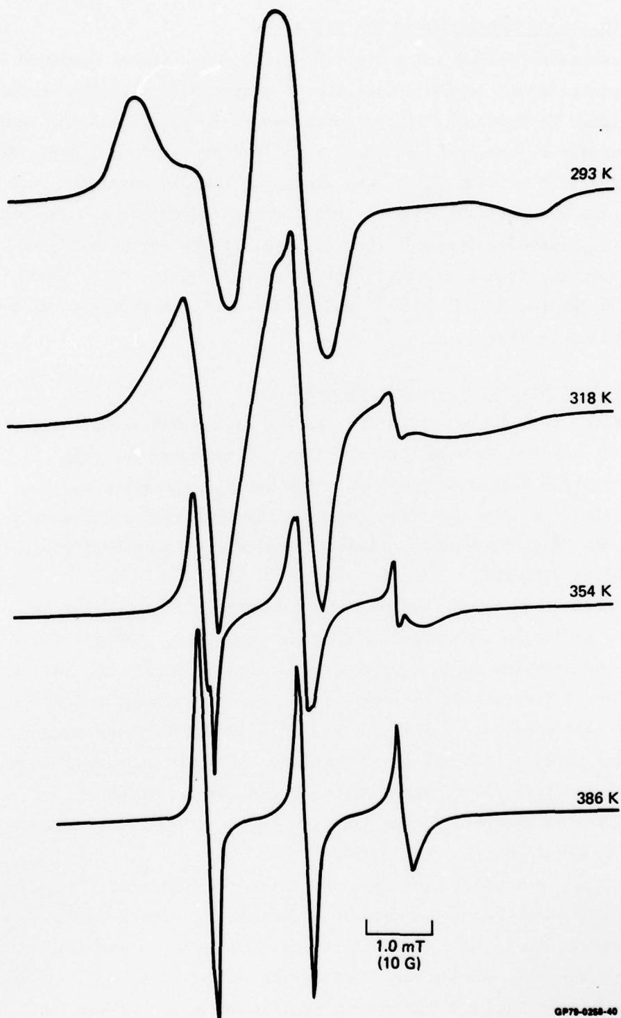
Figure 56 Spectra observed at 293 K, 318 K, 354 K, and 386 K from reverted TAMIN-labeled polyurethane (spin label II). A superposition of two fast-phase components can be observed in the 318 K, 354 K, and 386 K spectra.
