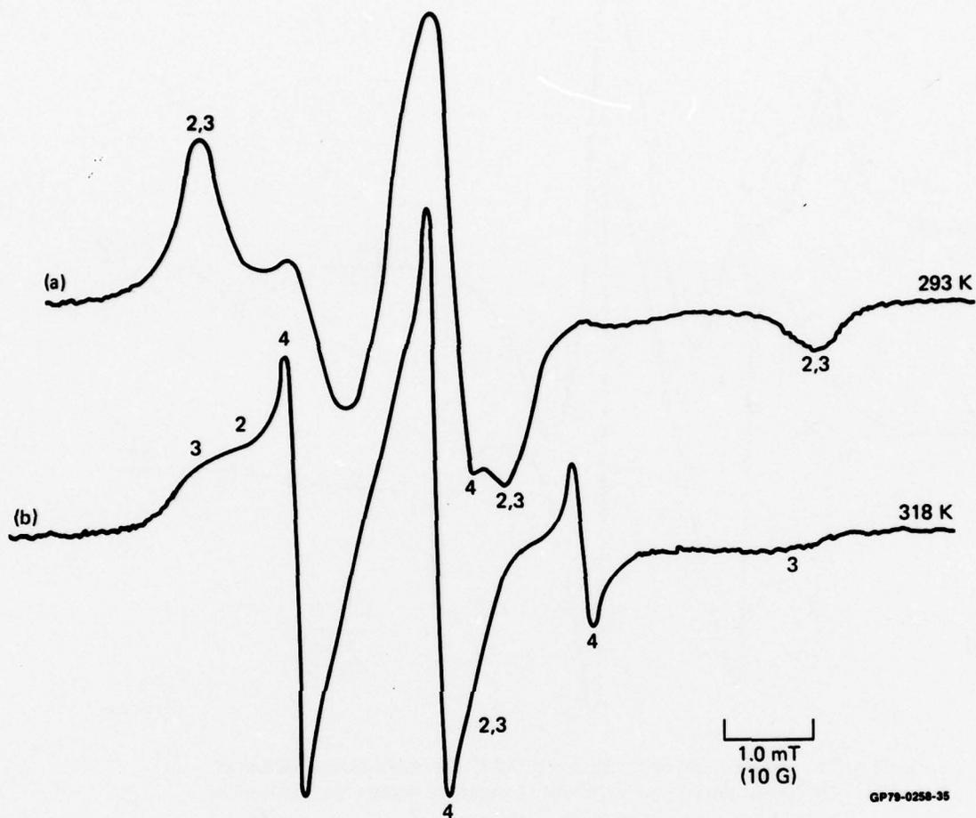
**Figure 5** The spectra observed at 293 K and 318 K after 72 h into the reaction of METAMIN with uncured DGEBA. Spectrum 2 denotes the spectrum of DGEBA end-labeled with METAMIN. Spectrum 3 denotes the spectrum of the spin-labeled quaternary salt. Spectrum 4 denotes the spectrum of the TEMPENE spin probe.
