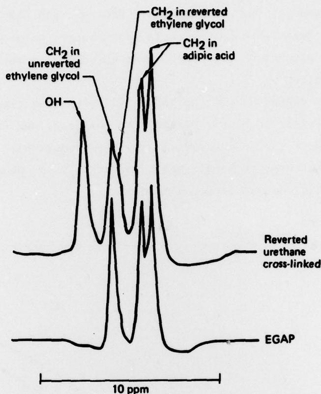
Figure 62 Room-temperature spectrum of extensively reverted polyester polyurethane.
