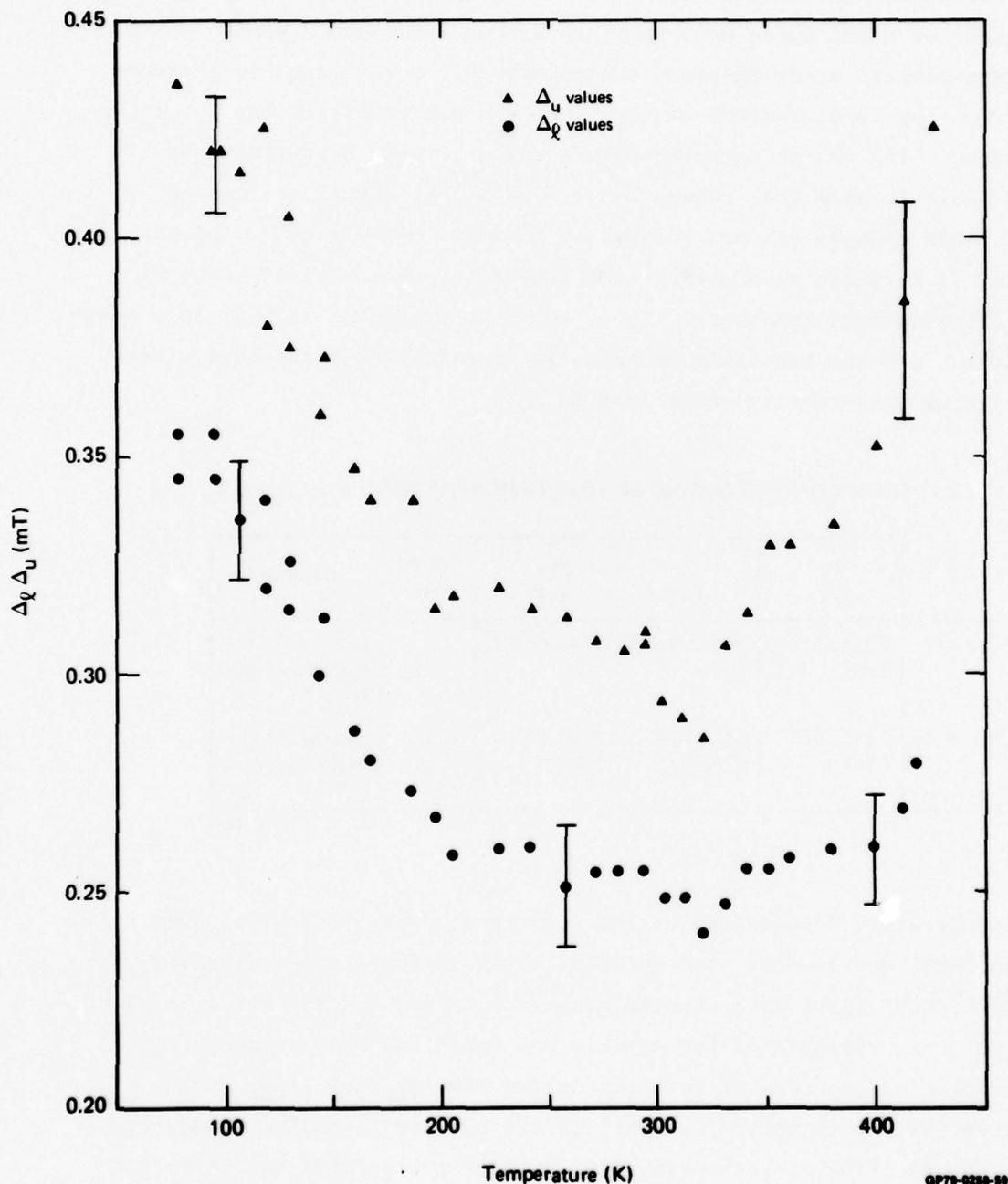
Figure 19 Temperature dependence of extrema widths  $\Delta_\rho$  and  $\Delta_u$  of TANOL in DGEBA cured with DETA (1:1 stoichiometry).
