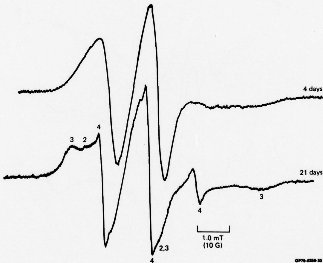
Figure 15 The spectra observed at 318 K after 4 days and 21 days into the reaction of TRIMETAMIN iodide with uncured DGEBA. Spectrum 2 denotes the spectrum of the TRIMETAMIN cation probe. Spectrum 3 denotes the spectrum of DGEBA end-labeled with DIMETAMIN. Spectrum 4 denotes the spectrum of the TEMPENE spin probe.
