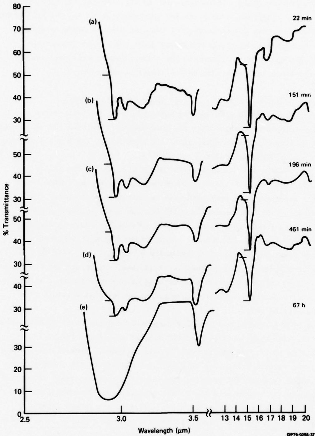
Figure 16 IR spectra observed at 293 K after (a) 22 min, (b) 151 min, (c) 196 min, (d) 461 min, and (e) 67 h following initial mixing of TAMIN with uncured DGEBA.
