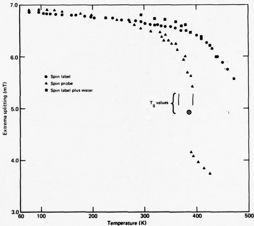
Figure 21 Temperature dependence of the extrema splitting ( $2\Delta_0$ ) for the spin-label bridging-group/quaternary-salt of TAMIN and the TANOL spin probe in DGEBA cured with DETA (1:1 stoichiometry). Also shown are data for the TAMIN sample containing 3.3 wt % water. Vertical bars indicate range of  $T_g$  values obtained using DSC and  $\otimes$  indicates the literature value for  $T_g$ .
