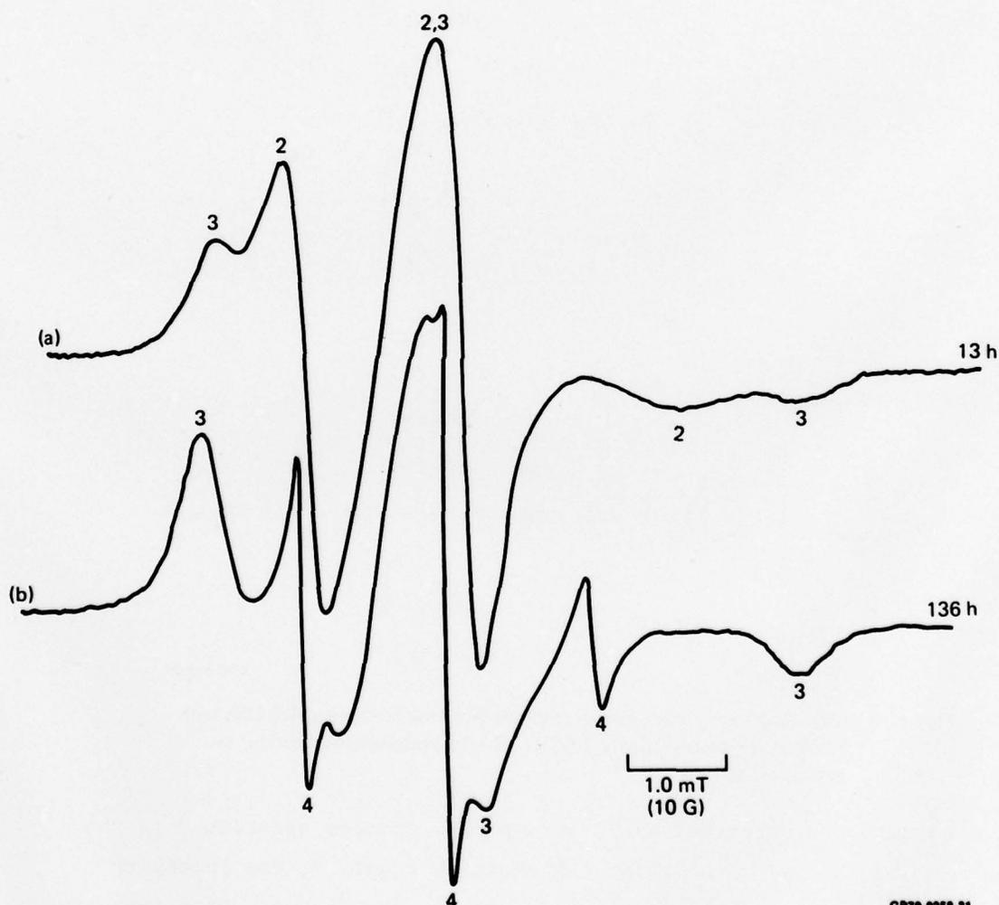
**Figure 11** The spectra observed at 318 K after 13 h and 136 h into the reaction of TAMIN with uncured DGEBA. Spectrum 2 denotes the spectrum of DGEBA end-labeled with TAMIN. Spectrum 3 denotes the spectrum of the bridging-group quaternary-salt. Spectrum 4 denotes the spectrum of the TEMPENE spin probe.
