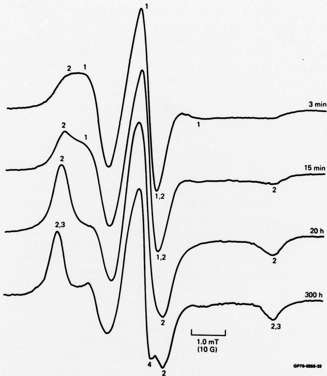
**Figure 3** Spectra observed at times 3 min, 15 min, 20 h, and 300 h into the reaction of METAMIN with uncured DGEBA. Spectrum 1 denotes the spectrum of the unreacted METAMIN spin probe. Spectrum 2 denotes the spectrum of DGEBA end-labeled with METAMIN. Spectrum 3 denotes the spectrum of the spin-labeled quaternary salt. Spectrum 4 denotes the spectrum of the TEMPENE spin probe.
