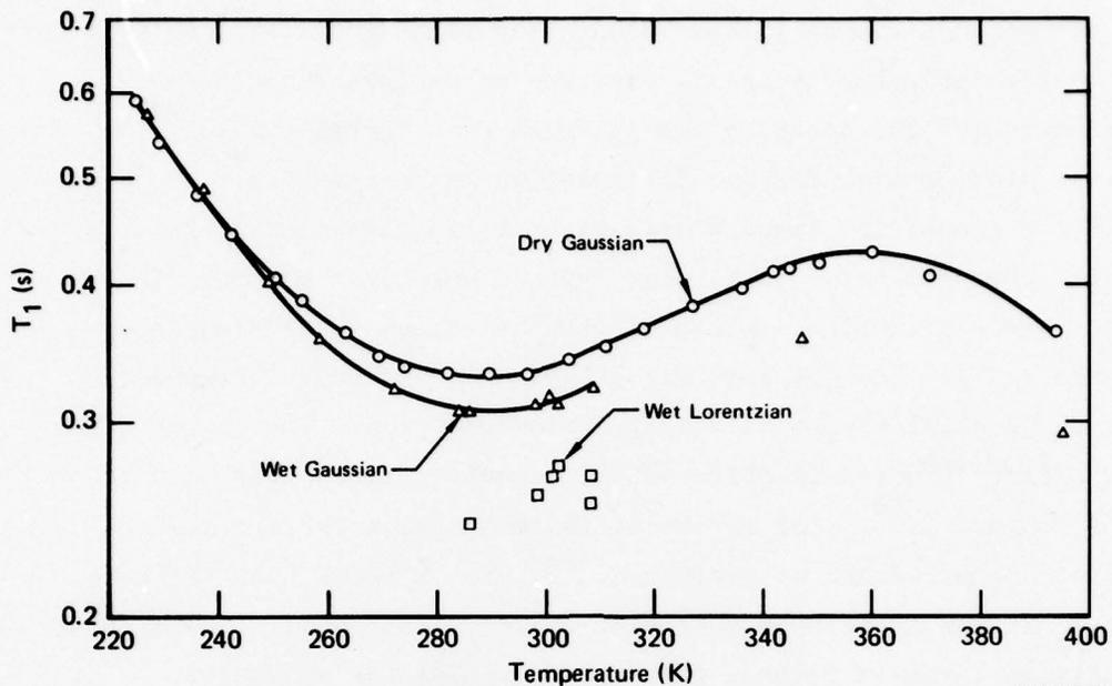
Figure 37 Spin-lattice relaxation times for wet and dry epoxy samples with 1:1 stoichiometry.
