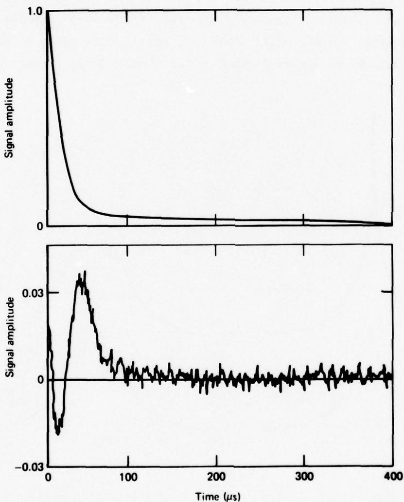
Figure 31 Room-temperature free-induction decay signal (a) for an epoxy resin sample containing 3.26 wt % water. In (b) the residual signal, after subtracting the Lorentzian signal,  $0.057 \exp(-t/176 \mu s)$ , and the Gaussian signal,  $0.943 \exp[-(t/17 \mu s)^2]$ , is shown.
