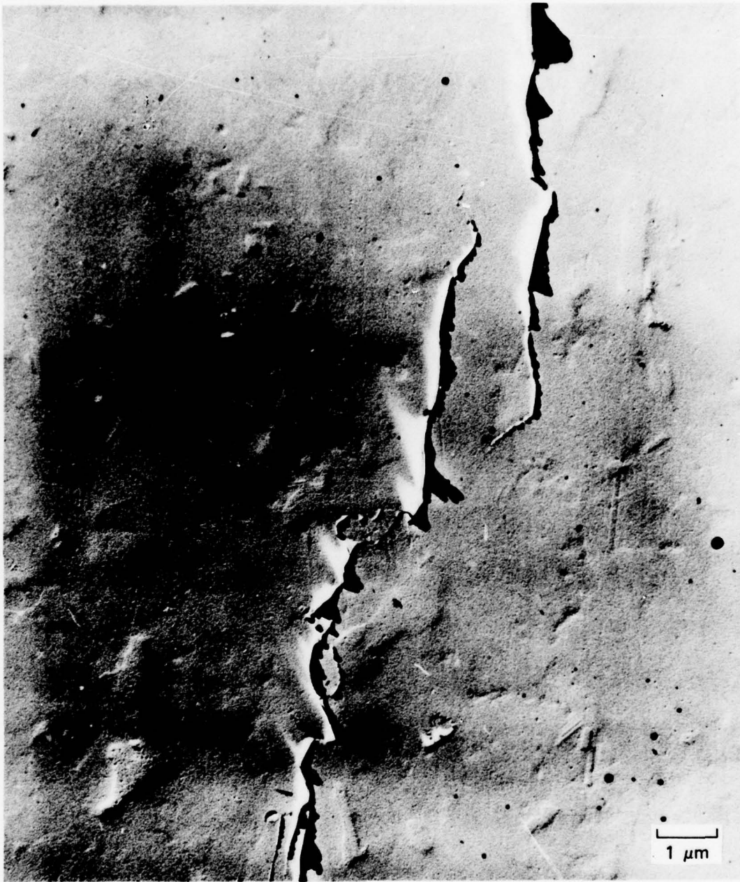
FIGURE 25 TYPICAL RING CRACKS IN HP \text{Si}_3\text{N}_4 PRODUCED BY QUASI-STATIC INDENTATION (Concluded)
