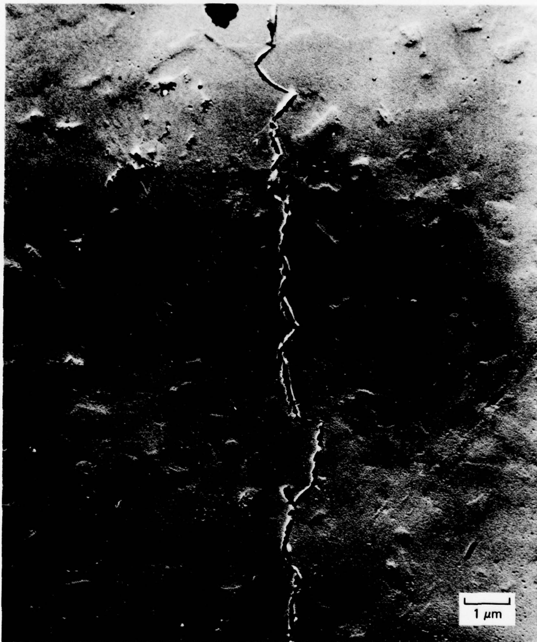
FIGURE 25 TYPICAL RING CRACKS IN HP \text{Si}_3\text{N}_4 PRODUCED BY QUASI-STATIC INDENTATION
