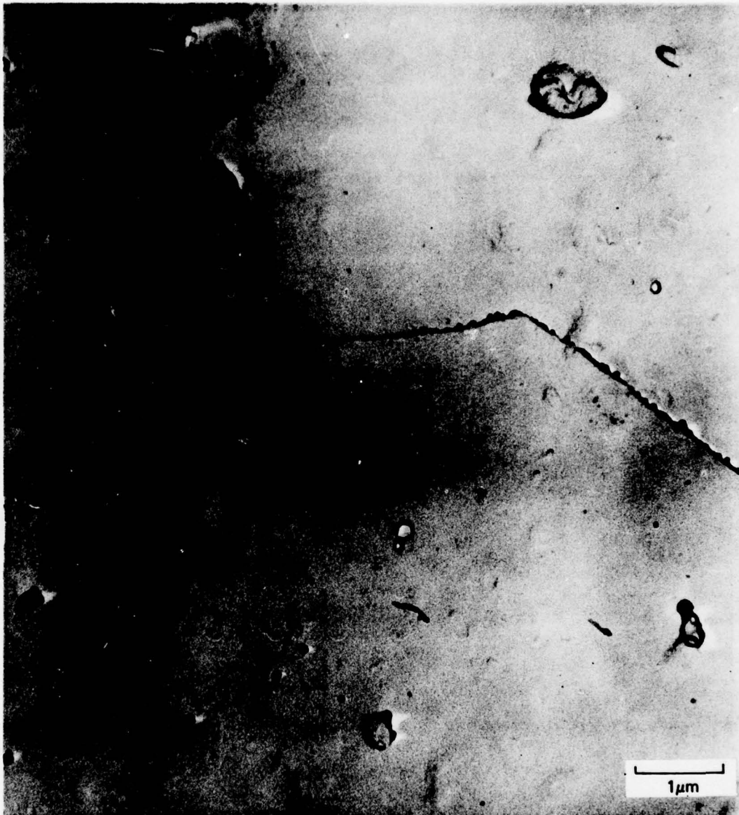
FIGURE 28 CRACK TIP OF A RADIAL SEGMENT (Shown in Figure 27) THAT VEERS TOWARD CONTACT CENTER
