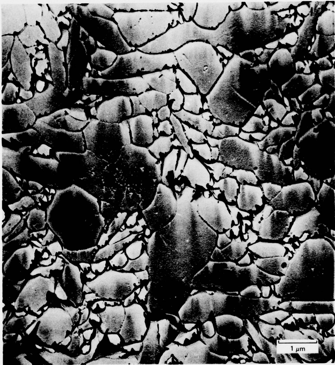
FIGURE 1 MICROSTRUCTURE OF HOT PRESSED SILICON NITRIDE
