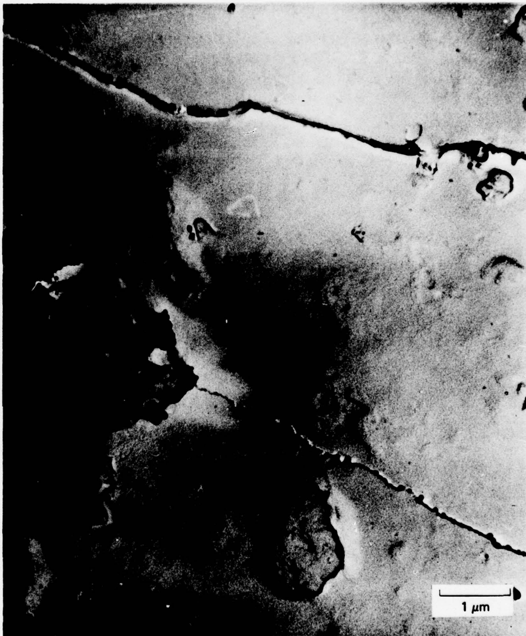
FIGURE 29 A RING CRACK IN RB \text{Si}_3\text{N}_4 PRODUCED BY QUASI-STATIC INDENTATION THAT TERMINATES AT A LARGE PORE
