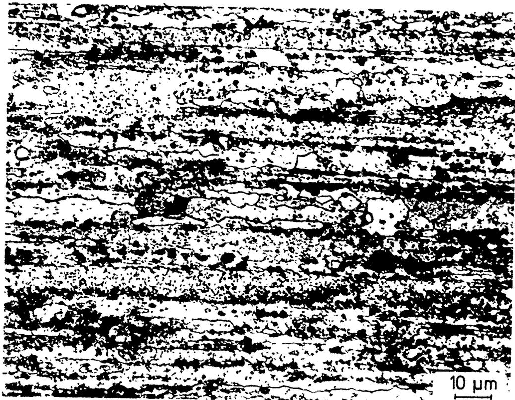
Figure 34 Representative optical micrographs of the grain structure of 2024-T3510 P/M 25:1 direct extrusions, with a 643 K extrusion-preheat, parallel to extrusion direction. (a) Barker's etchant, (b) electrolytically polished, and etched with 10 ml HF - 5 ml HNO<sub>3</sub> - 90 ml H<sub>2</sub>O (diluted).
