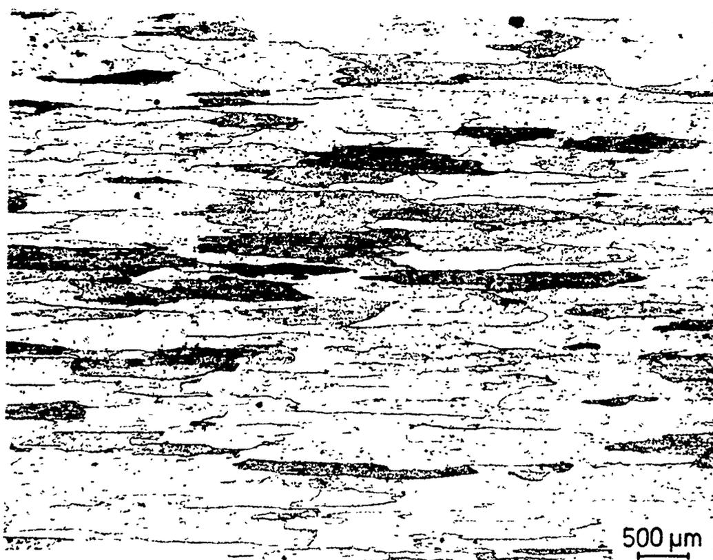
Figure 32 Representative optical micrographs of the grain structure of 2024-T3510 I/M 25:1 direct extrusions etched with 10 ml HF - 5 ml HNO<sub>3</sub> - 90 ml H<sub>2</sub>O : (a) alloy A (commercial product) parallel and perpendicular to the extrusion direction, also typical of alloy B (b) control alloy C (643 K extrusion-preheat) parallel to the extrusion direction.
