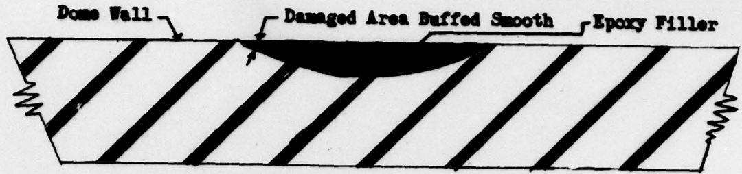
a. REPAIR OF MINOR SURFACE DAMAGE
