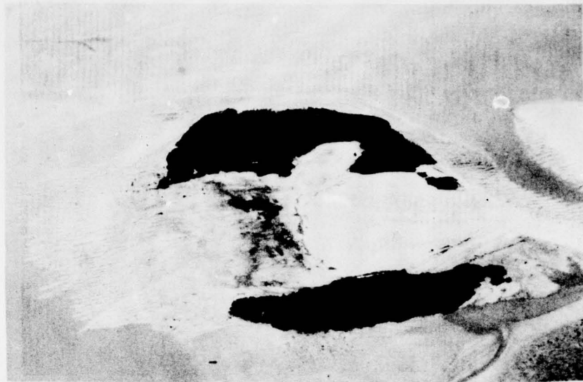
a. The site was formed by grading this sandy dredged material island to achieve a 2-ha intertidal area
