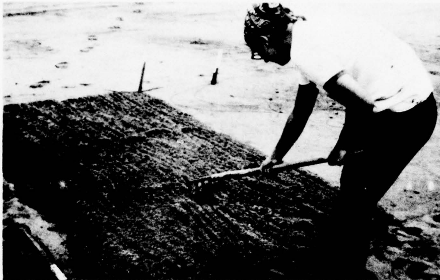
Figure 28. Fertilizing sandy test plots at the Buttermilk Sound site before planting. Fertilization is seldom necessary on fine-textured material but may be desirable on sandy dredged material
