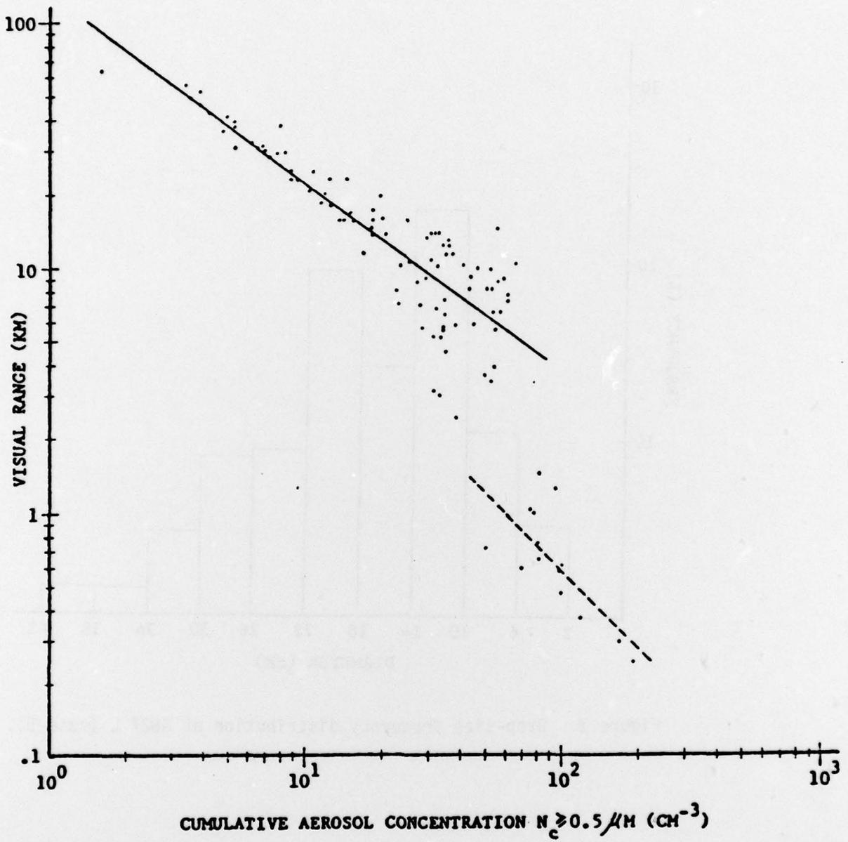
Figure 4. Visual range versus cumulative aerosol concentration.
