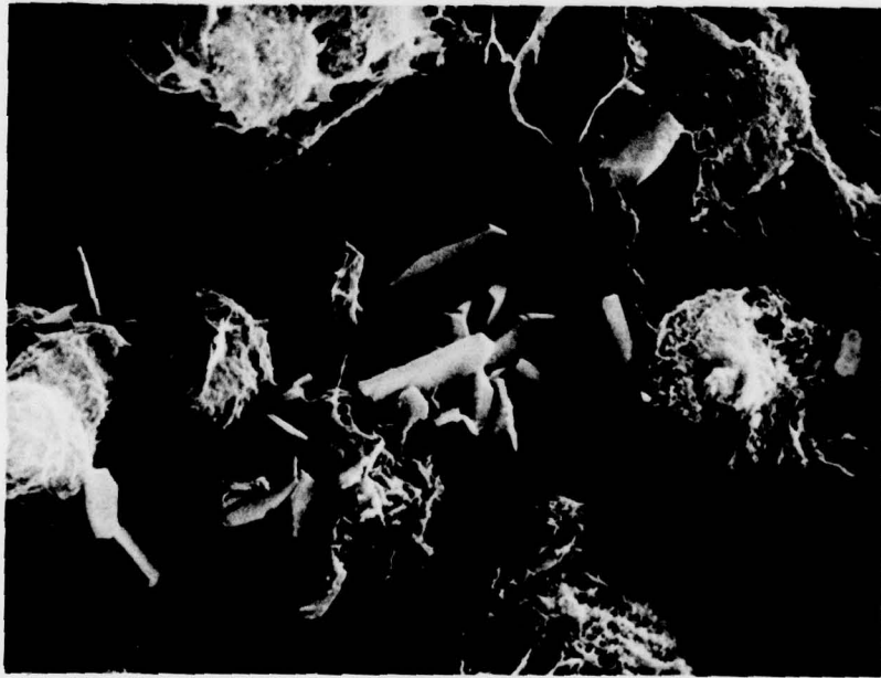
Figure 4. Grout samples E, X2300. Upper sample was freeze dried following vacuum drying while bottom one was not. There is no detectable effect of this difference. These are enlargements of the areas shown in Figure 3.
