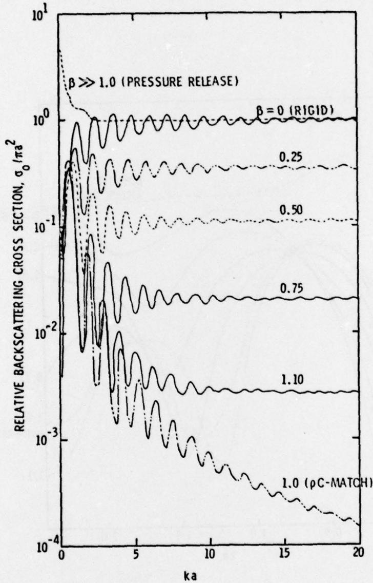
Figure 1 - Backscattering cross section curves for various values of  $\beta$  and for  $0.2 \leq ka \leq 21$ .
