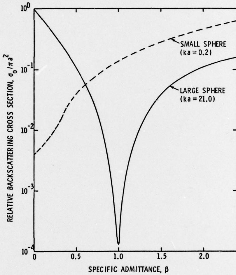
Figure 3 - The variation of the backscattering cross section with  $\beta$  for both large and small spheres.
