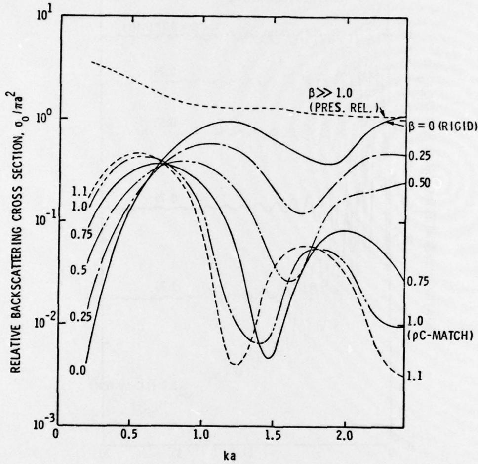
Figure 2 - Backscattering cross section curves for various values of  $\beta$  and for  $0.2 \leq ka \leq 2.4$ .
