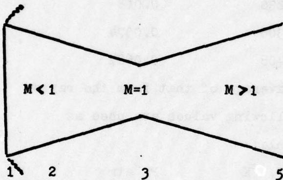
Figure 1. Entrance Shock for Starting Ramjet-Subcritical Condition
