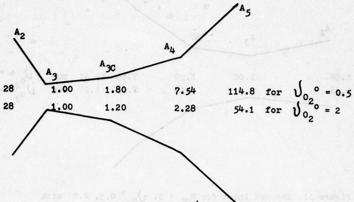
Figure 13. Shock Expelled for  $M_\infty = 5$ ,  $v_{0_2}^0 = 0.5, 2$  with Area Relationships
