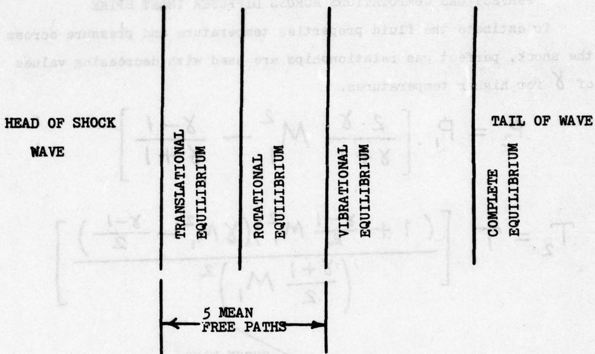
Figure 4. Internal Modes of Energy of Diatomic Oxygen and Nitrogen Showing Regions of Relaxion
