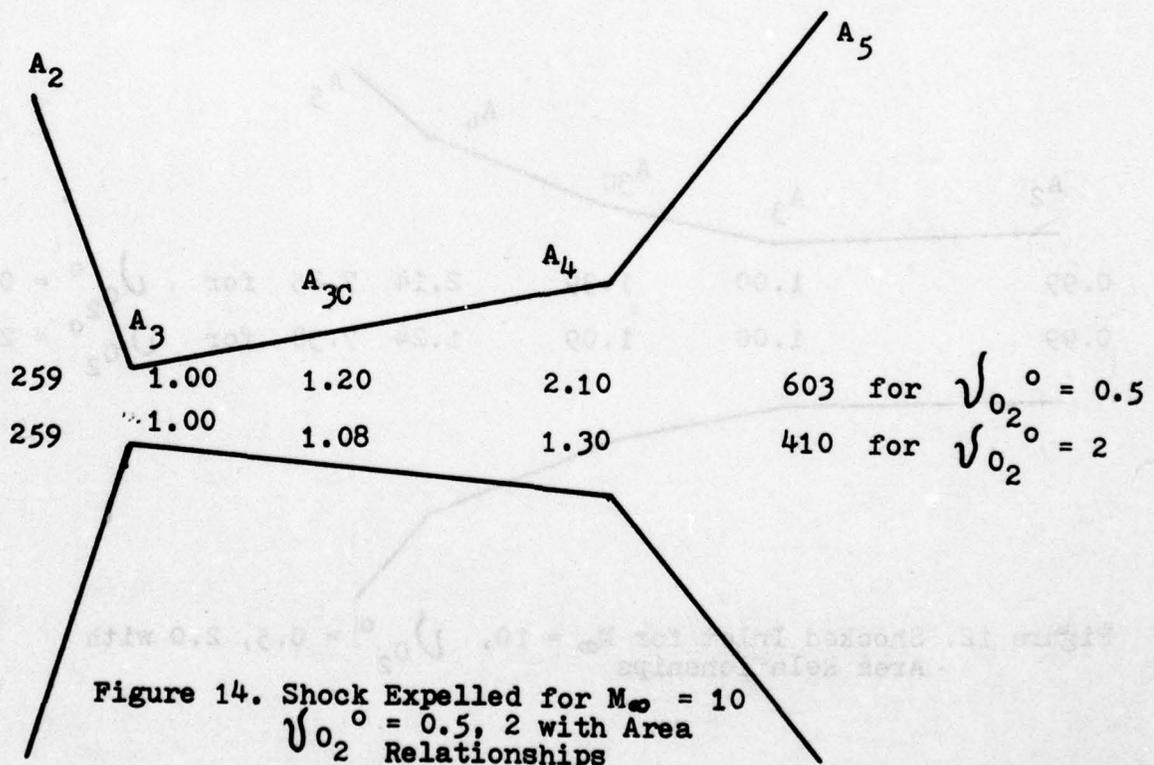
Figure 14. Shock Expelled for  $M_\infty = 10$ ,  $v_{0_2}^0 = 0.5, 2$  with Area Relationships
