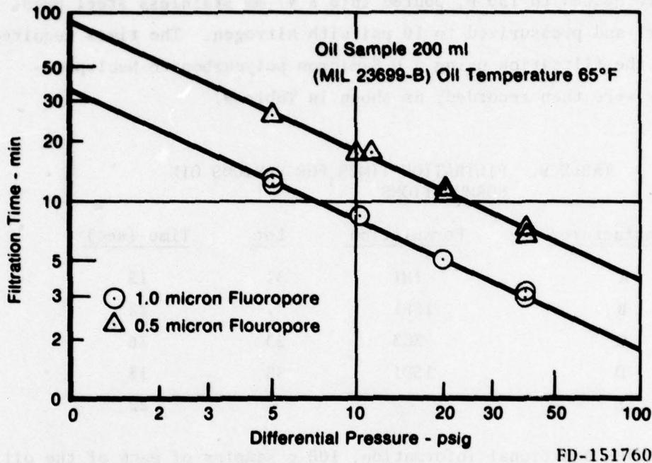
Figure 11. Oil Filtration Time vs Applied Pressure
