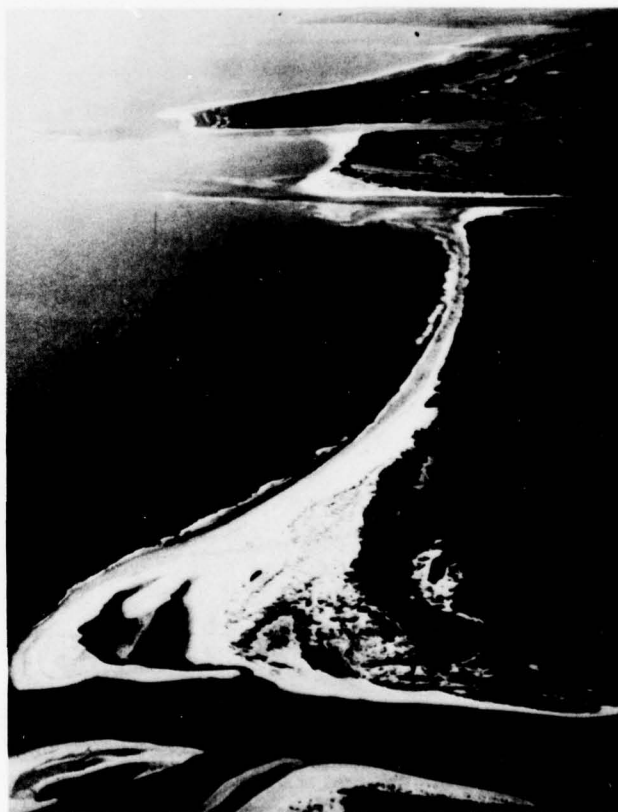
Figure 14. Oblique IR aerial photo of Capers Island looking southeast. Note erosion of antecedent beach ridges which has left a forest of driftwood along portions of the beach.
