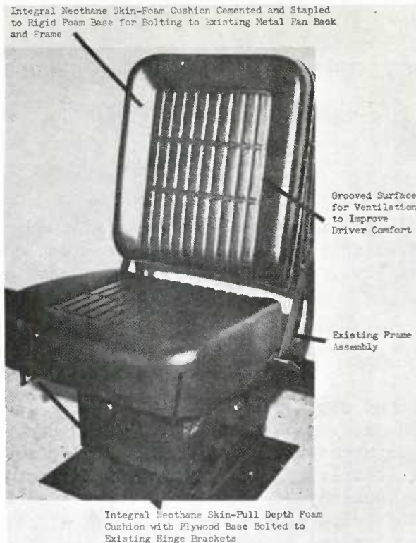
Figure 1 - Proposed Driver Seat Assembly for 800 Series 5-Ton Vehicle
