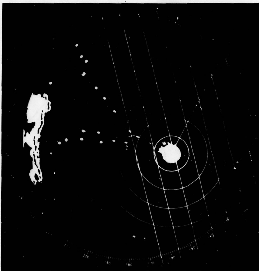
Figure 2A. Radar Screen Photograph showing displaced positions, after three hours, of floats deployed in Western Wakasa Bay. Time: 1430 hours on 9 August 1978. North is at top of the photograph. The rings are one-half mile range markers. The lines of floats radiating in the 320^{\circ} - 330^{\circ} sector and in the 260^{\circ} - 280^{\circ} sector were in lines of slicks. (Photography courtesy Professor H. Kawai and The Geophysical Institute, Kyoto University.)
