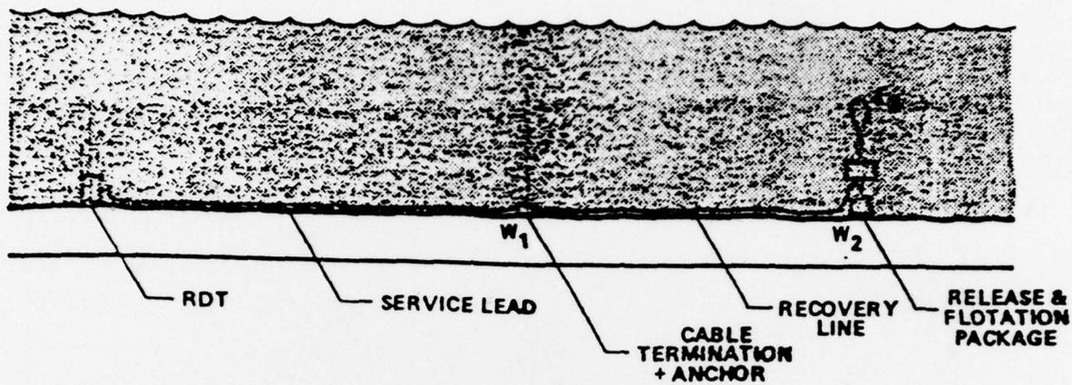
Figure A-2. Service lead and recovery line assembly arrangement installed on the ocean floor.
