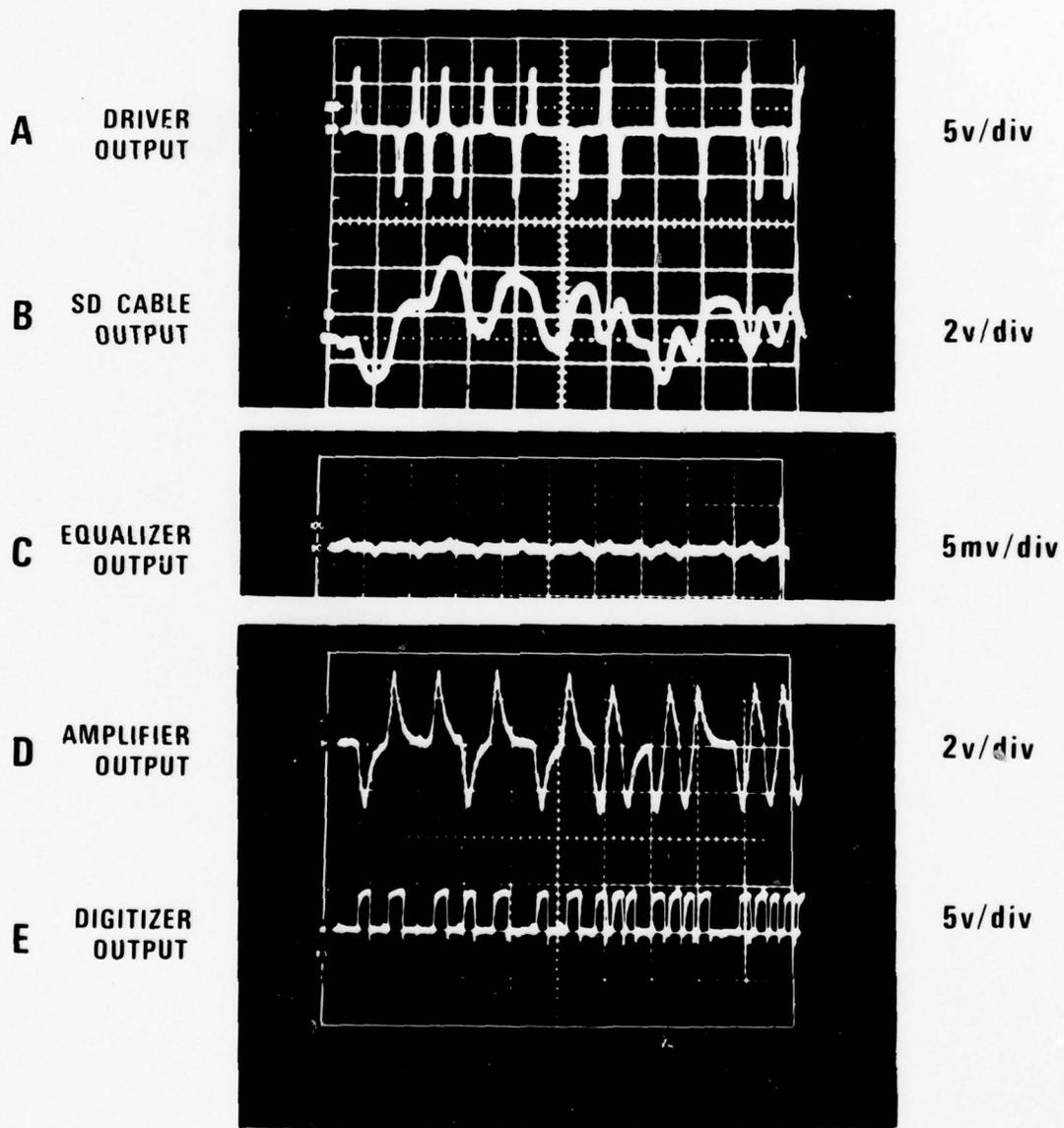
Figure 9. Telemetry waveforms.
