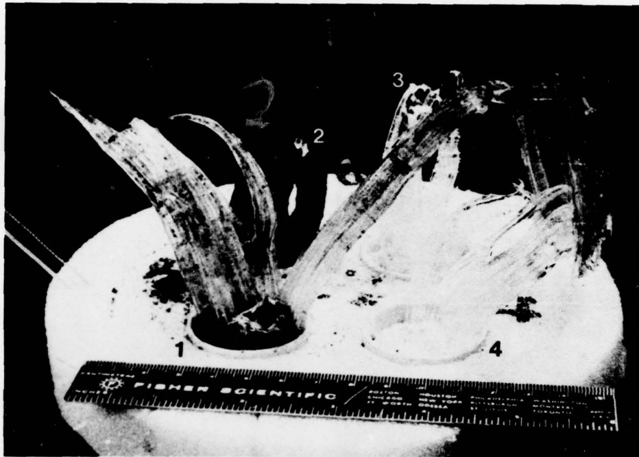
Figure A5. 1. Kanto loam #1: 100-mm multiple ice columns (older piece dangling at right). 2. Kanto loam #1 + 0.15% Natrosol: 30 -mm heave (behind #1). 3. Celite: 58-mm multiple ice columns. 4. Celite + 0.25% Natrosol: 60-mm multiple ice columns.
