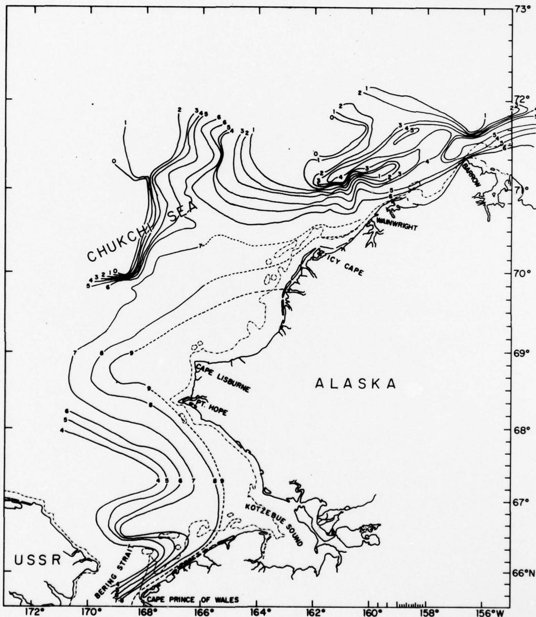
Figure 20. Isotherms of maximum temperature in the water column for MIZPAC 78. Temperatures are in degrees centigrade ( $^{\circ}\text{C}$ ). The dashed line paralleling the coast represents the 10 fathom curve.
