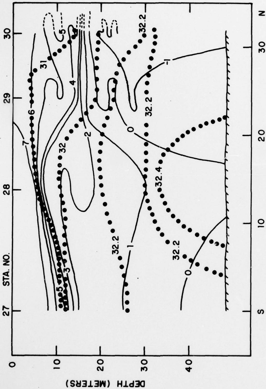
Figure 12. Temperature and salinity cross section No. 4.
