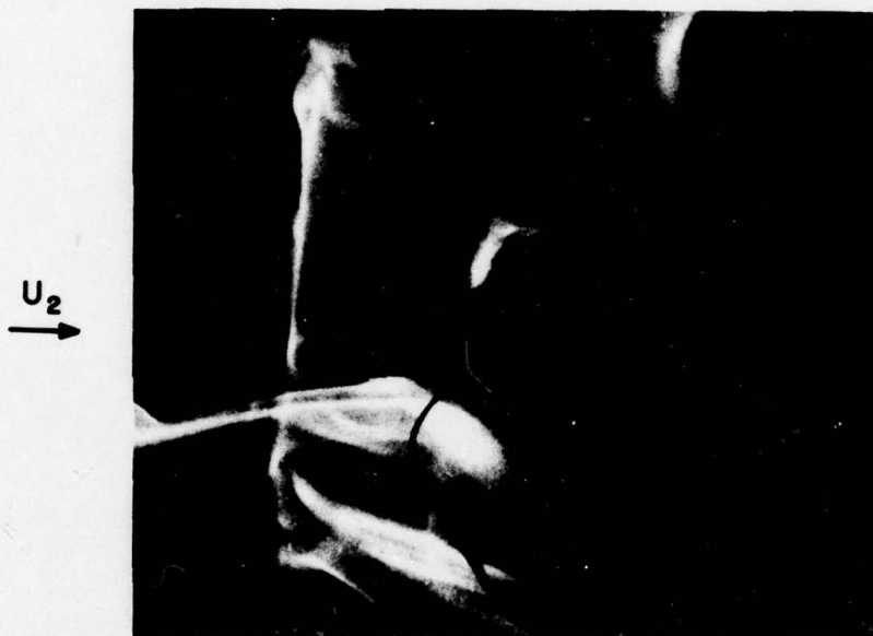
Fig. 2. Side view of a stretched cross-vortex tube near the leading edge of a symmetric NACA 65-010 profile at zero angle of attack and at a profile-chord Reynolds number of 2 \times 10^4 ; f/5.6 , 1/30 s; U_2 is the oncoming total velocity.
