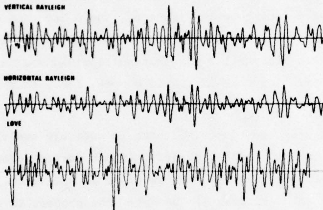
Figure 9 The surface wave as reconstructed from the synthetic record of Figure 8 by the single-station maximum-likelihood detector.
