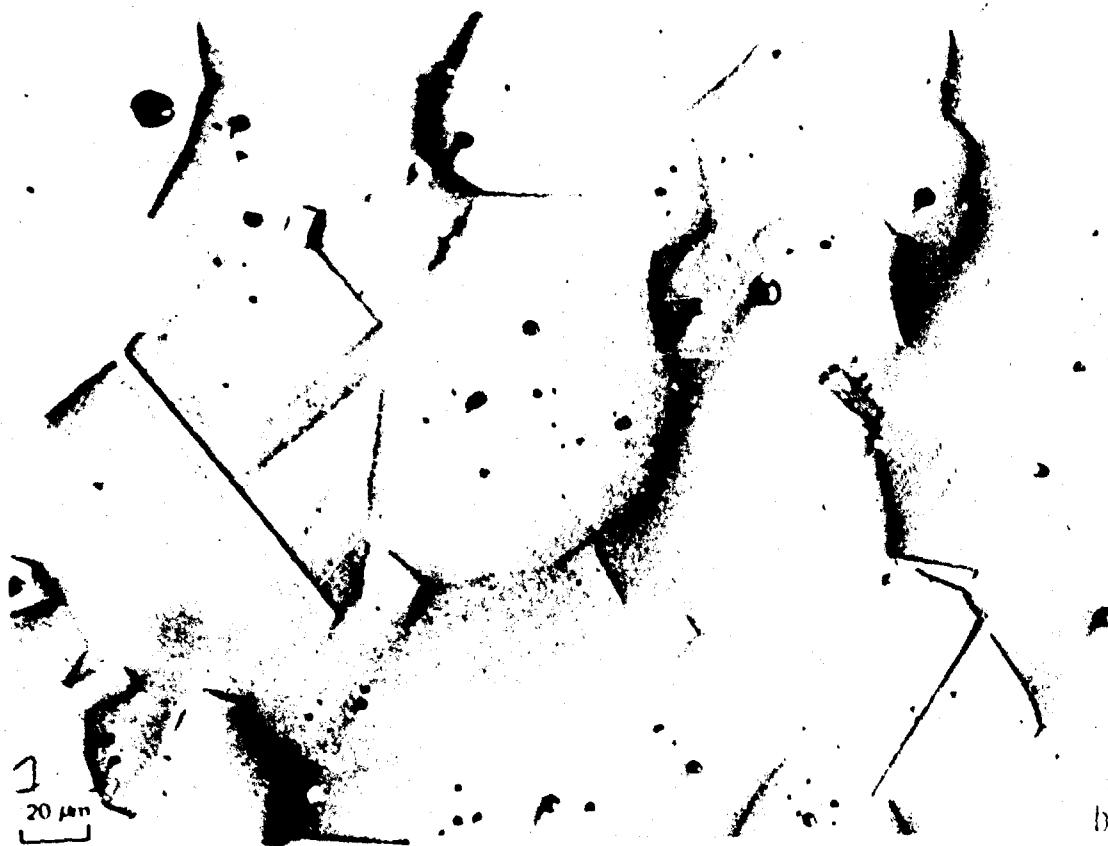
Figure 6. Microstructures of single-phase cubic aluminum oxynitride spinel; T = 1975 C; 30 mole % AlN; 1 hour.
