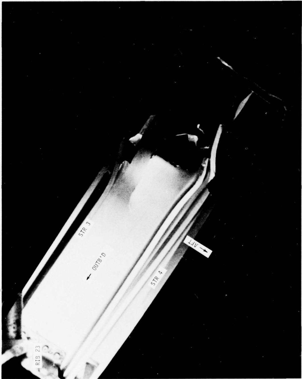
Figure 18. Inside of Wing Upper Cover Between BL 0 and LBL 23
