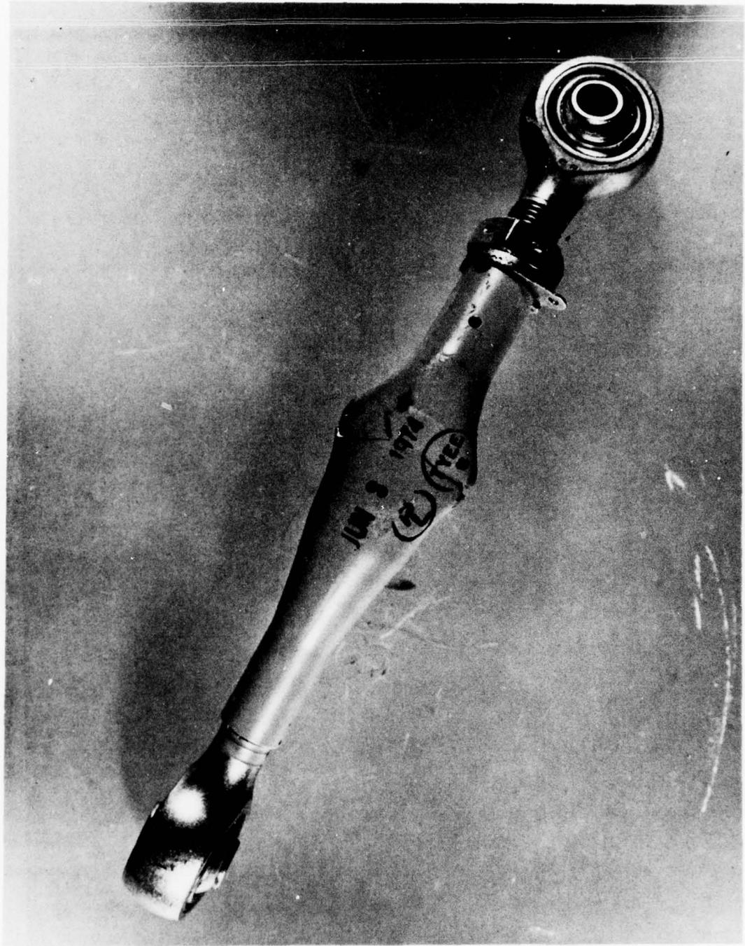
Figure 19. Failed Yaw Output Pushrod - Part No. 160C123005
