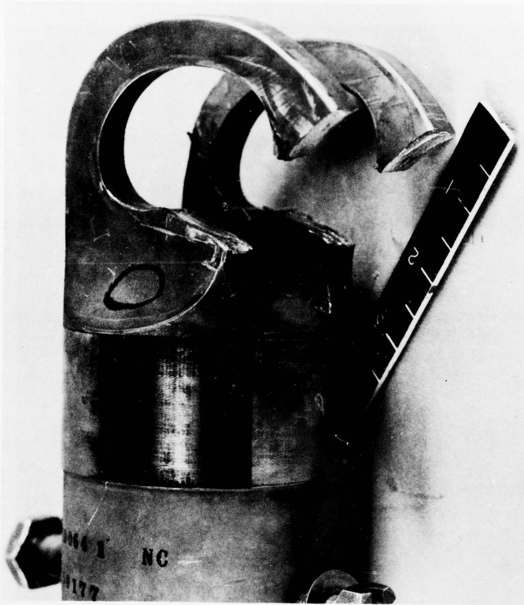
Figure 34. Drag Strut Pick-up Lugs After Failing Load Test
