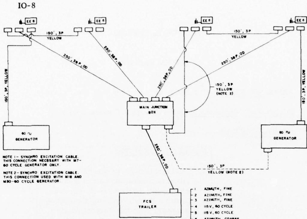
NOTE 1 - SYNCHRO EXCITATION CABLE. THIS CONNECTION NECESSARY WITH M7-60 CYCLE GENERATOR ONLY.
