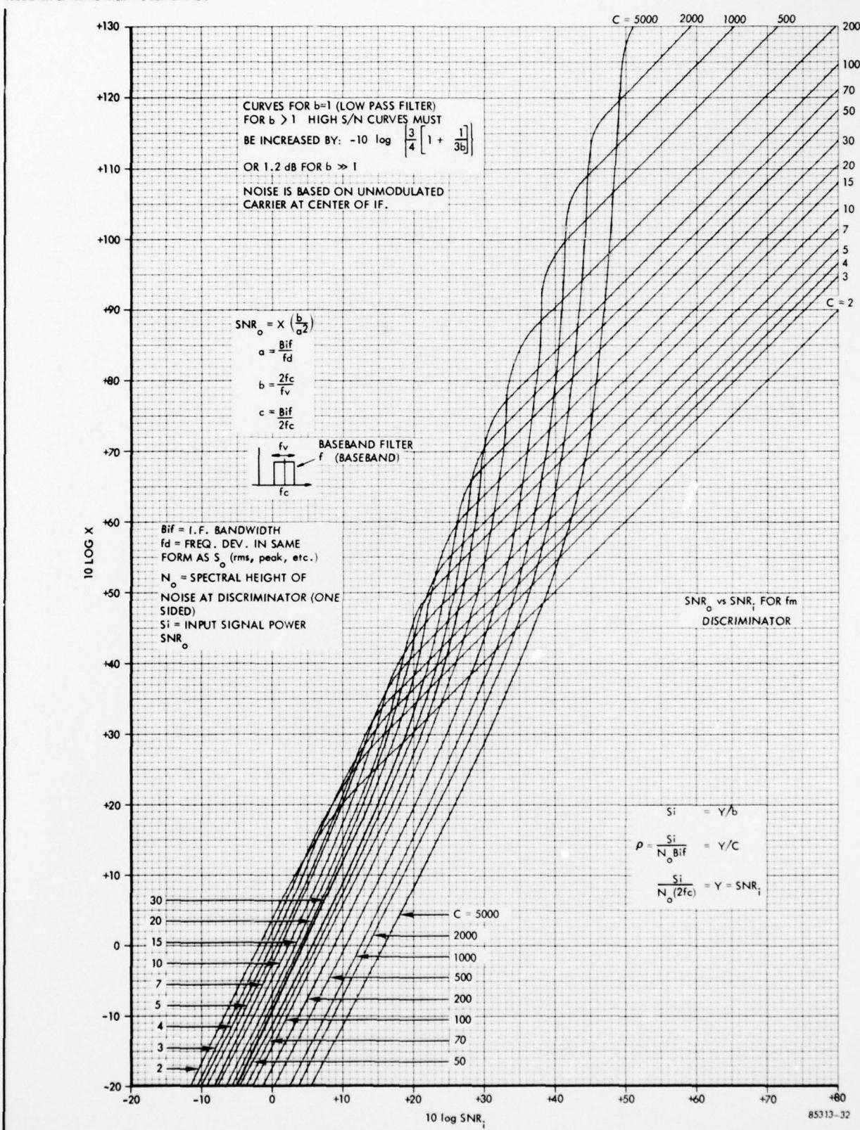
FIGURE 5-1  $\text{SNR}_o$  VS.  $\text{SNR}_i$  FOR FM DISCRIMINATOR
