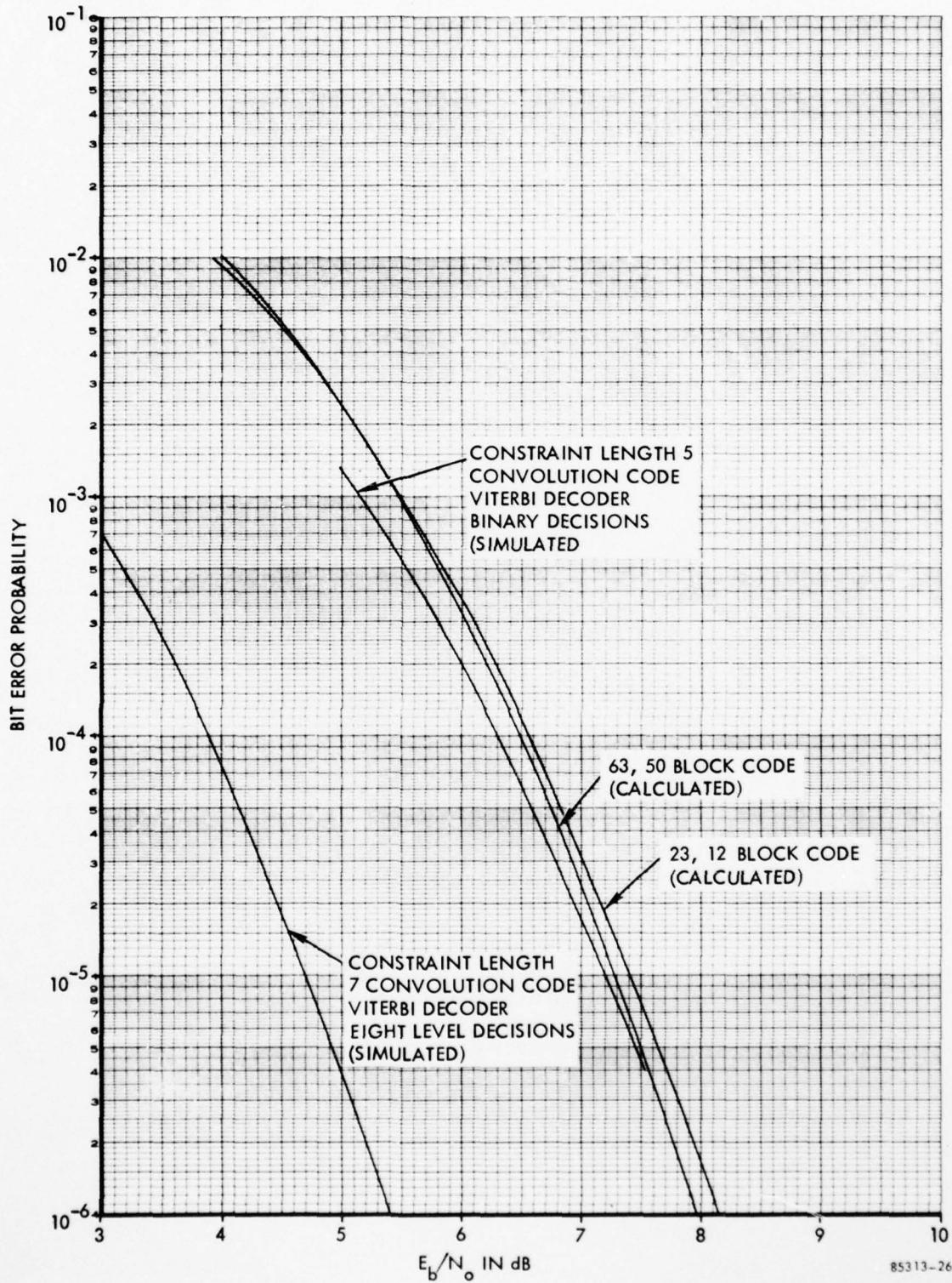
FIGURE 5-3 BIT ERROR RATE VS.  $E_b/N_o$  FOR
