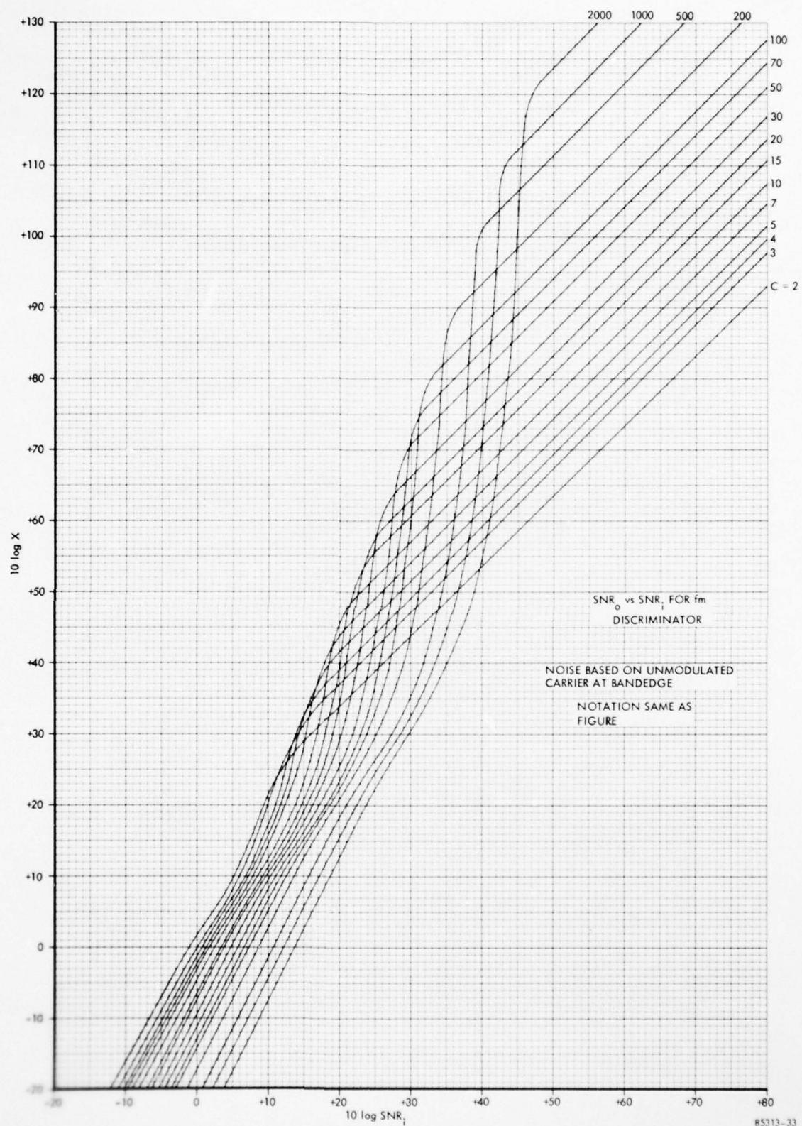
FIGURE 5-2  $\text{SNR}_o$  VS.  $\text{SNR}_i$  FOR FM DISCRIMINATOR
