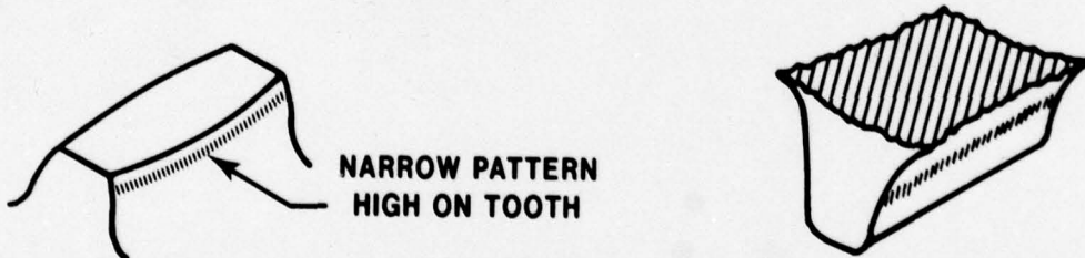
UNSATISFACTORY CONTACT PATTERN — PRESSURE ANGLE MISMATCH
