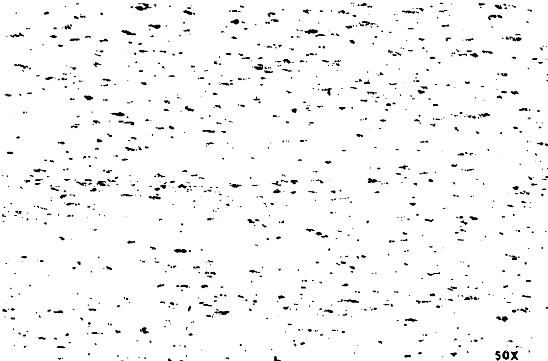
Figure 2-5. (a) Macrograph Showing a Transverse Section Through a Large Blister. (b) As-polished Micrograph in the Vicinity of the Large Blister in (a). The small black areas are fine porosity.
