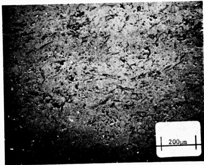
Fig. 4. Section through a composite containing 20 volume % Al 2 O 3 fibers.
