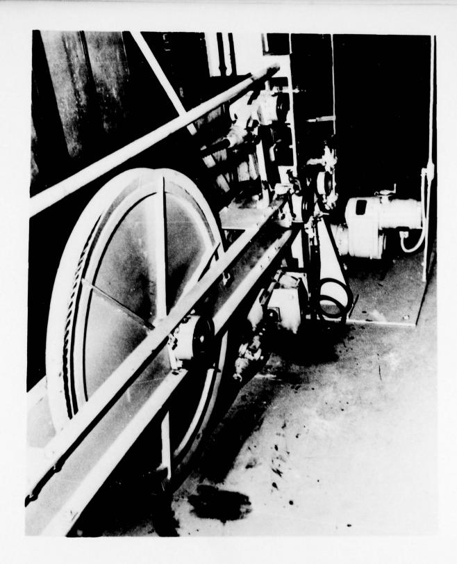
FIGURE 1 MCKLERNAN-TERRY FAIRING COLLAR TEST MACHINE. LEFT FRONT ANGLE VIEW PHOTO 121198-1
