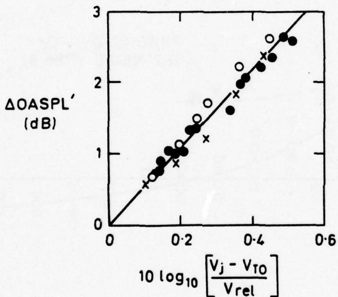
**FIG. 6 JET NOISE REDUCTIONS IN FLIGHT FOR VARIOUS NOZZLE SIZES**
