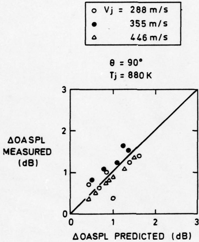
FIG. 8 NOISE REDUCTIONS IN FLIGHT FOR A HEATED JET
