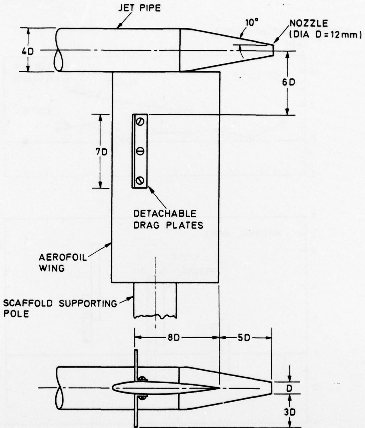
**FIG. 38 A DIAGRAM OF THE SPINNING RIG MODEL**
