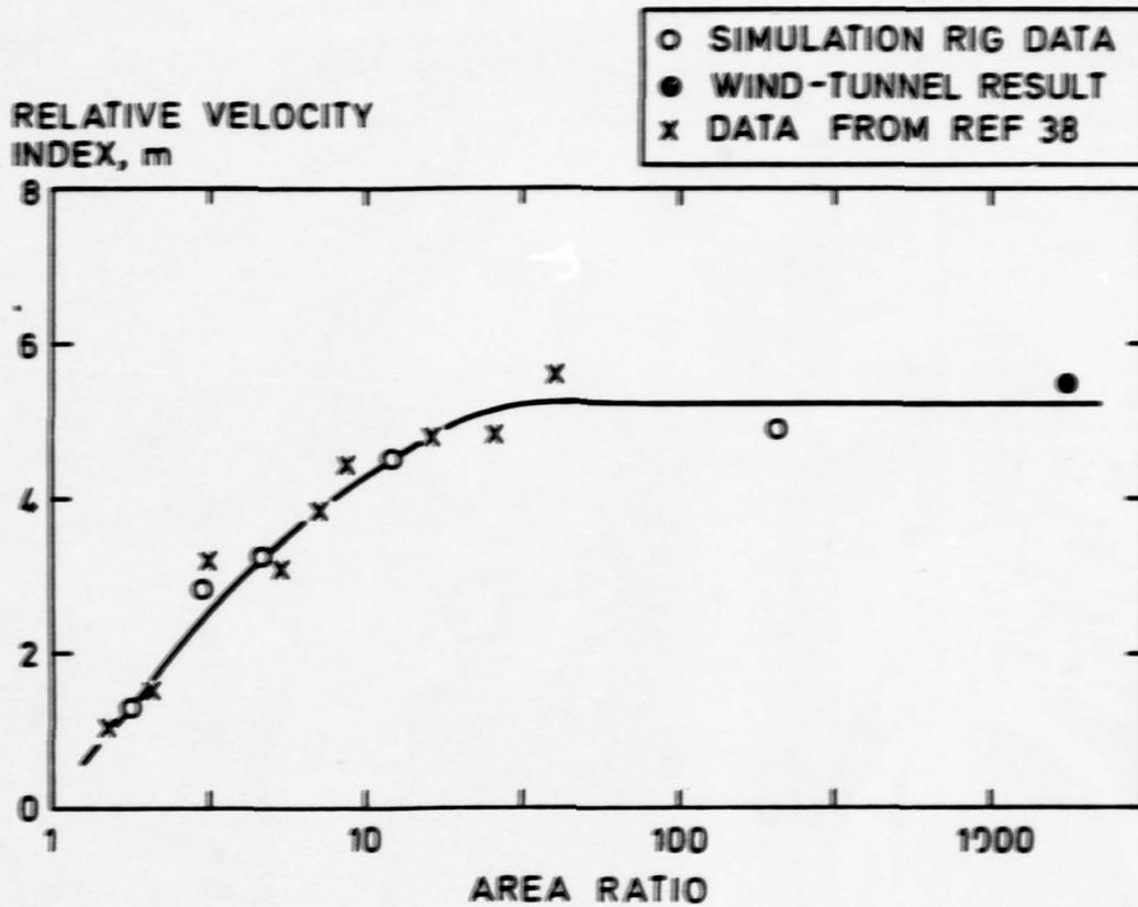
FIG. 16 THE DEPENDENCE OF THE RELATIVE VELOCITY INDEX AT 90° ON AREA RATIO
