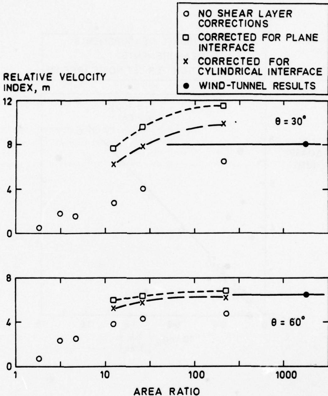
FIG. 17 THE EFFECT OF SHEAR LAYER CORRECTIONS ON REAR ARC DATA
