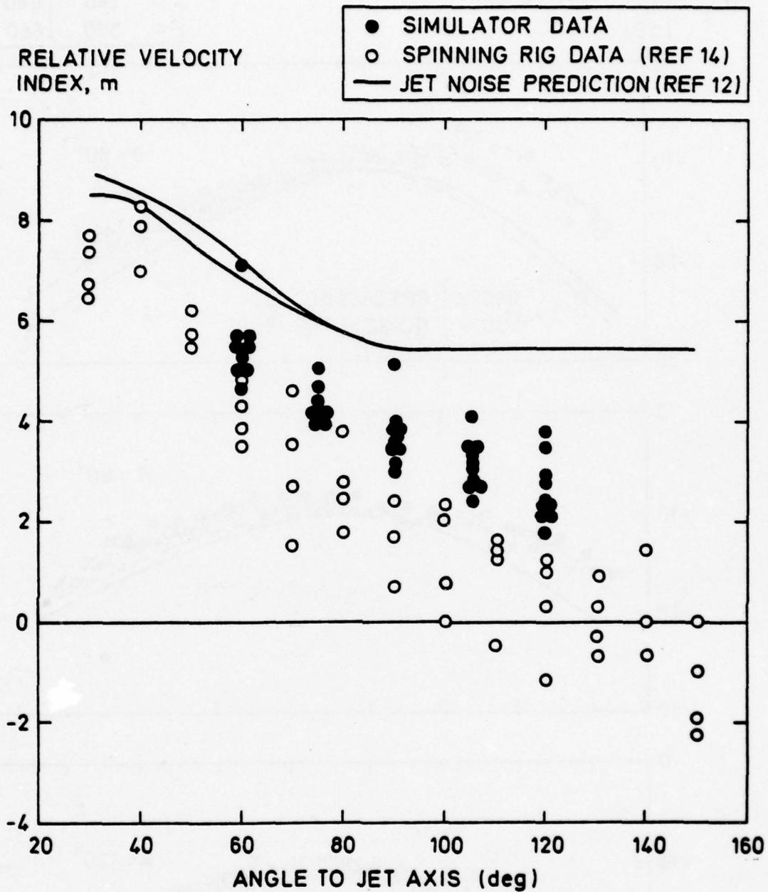
FIG. 28 A COMPARISON OF RESULTS FROM THE SPINNING RIG AND ITS SIMULATOR
