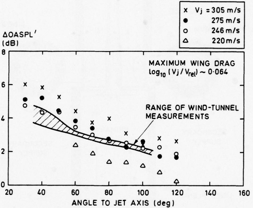
FIG. 13 A COMPARISON OF SPINNING RIG AND WIND-TUNNEL RESULTS FOR THE HSA NOZZLE
