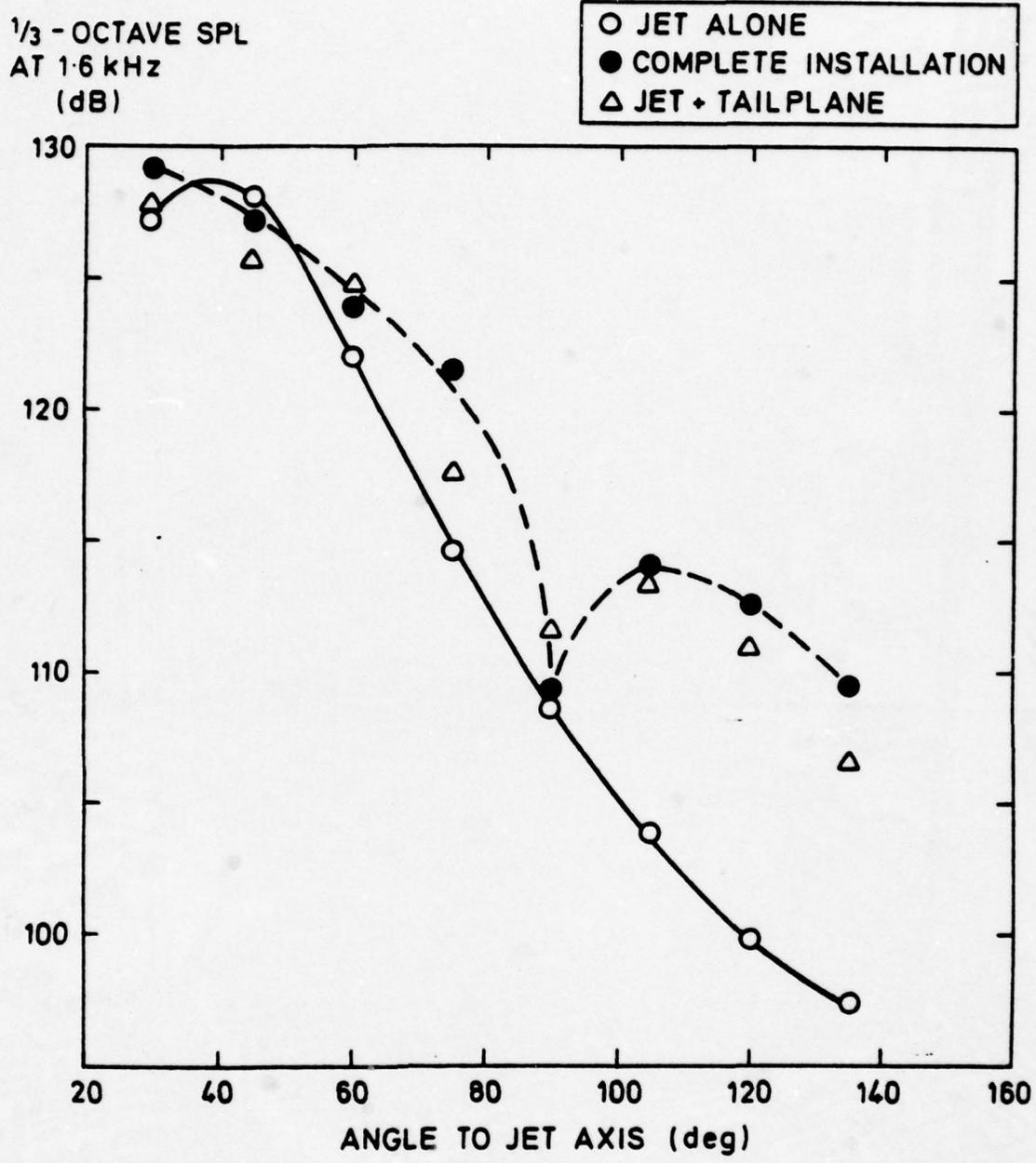
FIG. 31 POLAR DIRECTIVITY OF THE INTERNAL NOISE TONE WITH AND WITHOUT THE HS125 MODEL
