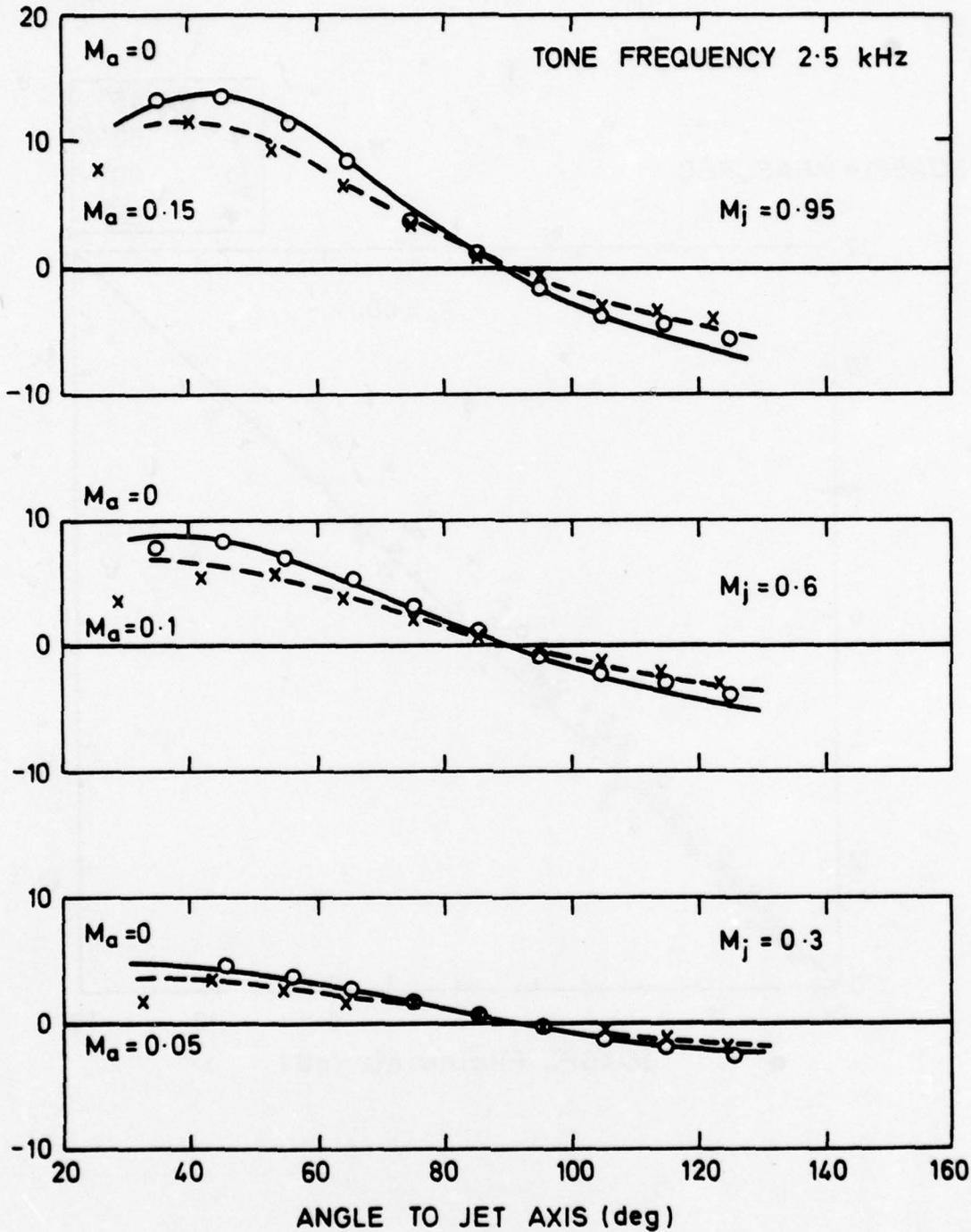
**FIG. 20 THEORETICAL AND EXPERIMENTAL FLIGHT EFFECTS ON INTERNAL NOISE**
