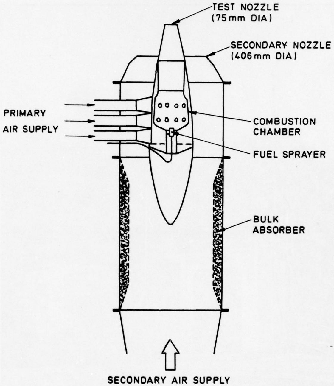
FIG. 25 THE SPINNING RIG SIMULATOR
