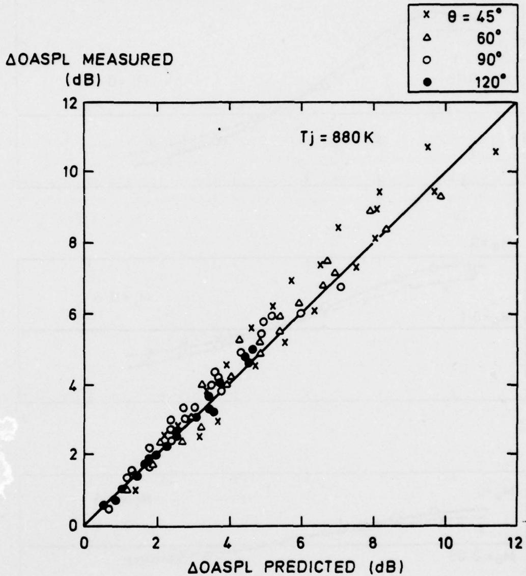
FIG. 19 A COMPARISON BETWEEN MEASURED AND PREDICTED CHANGES IN OASPL FOR HEATED JETS
