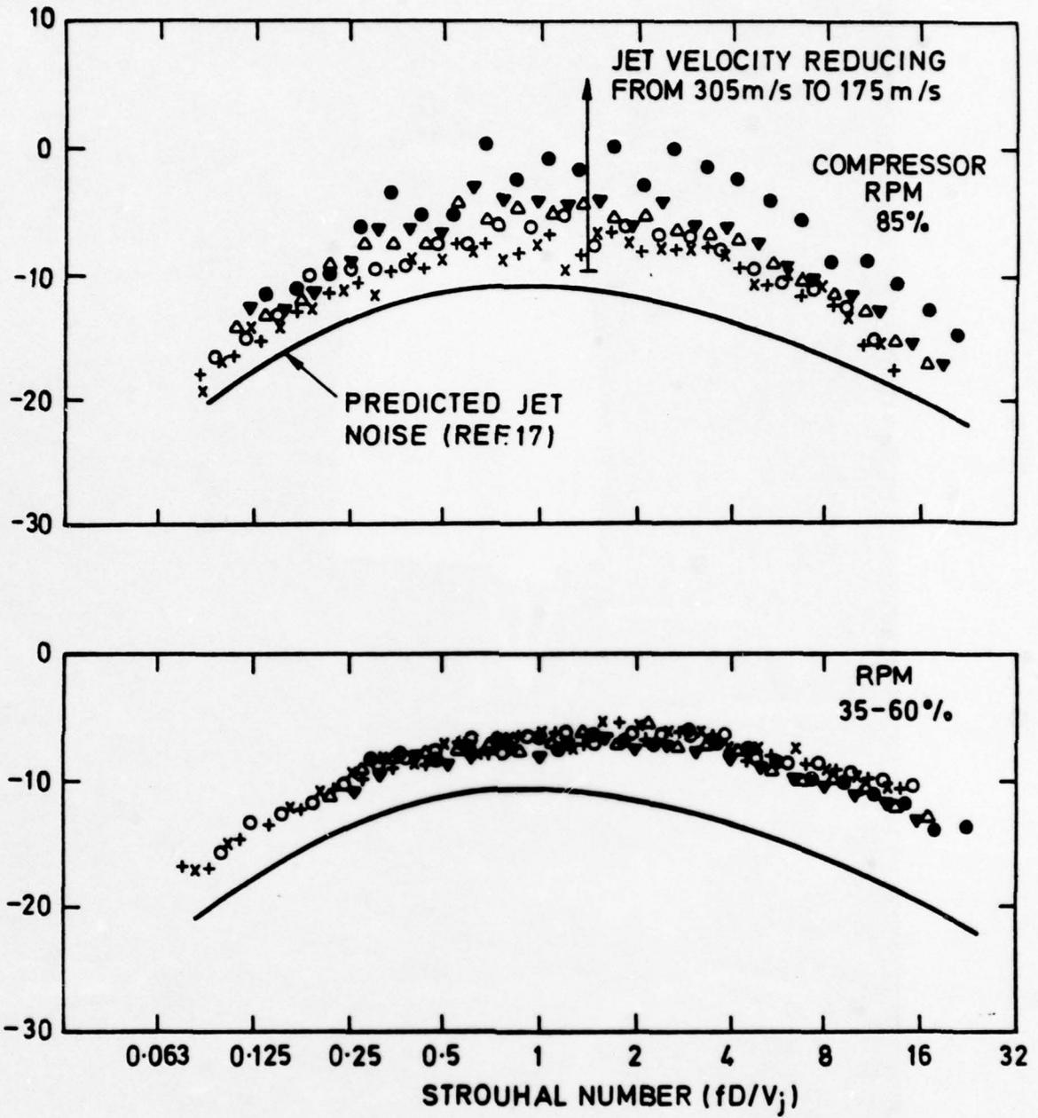
FIG. 12 STATIC SPECTRA AT 90° FROM THE HSA NOZZLE ON THE SPINNING RIG
