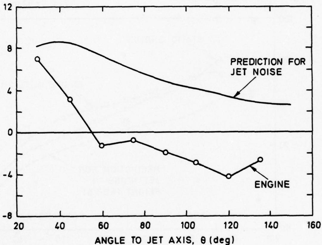
FIG. 2 CHANGES OF EXHAUST NOISE IN FLIGHT
