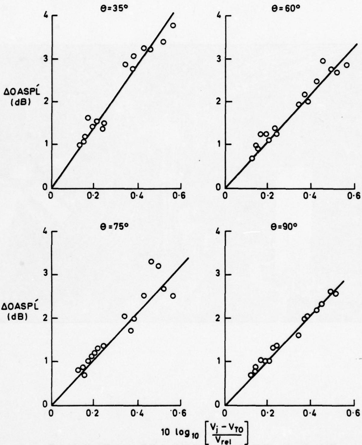
**FIG. 4 NOISE REDUCTIONS IN FLIGHT
