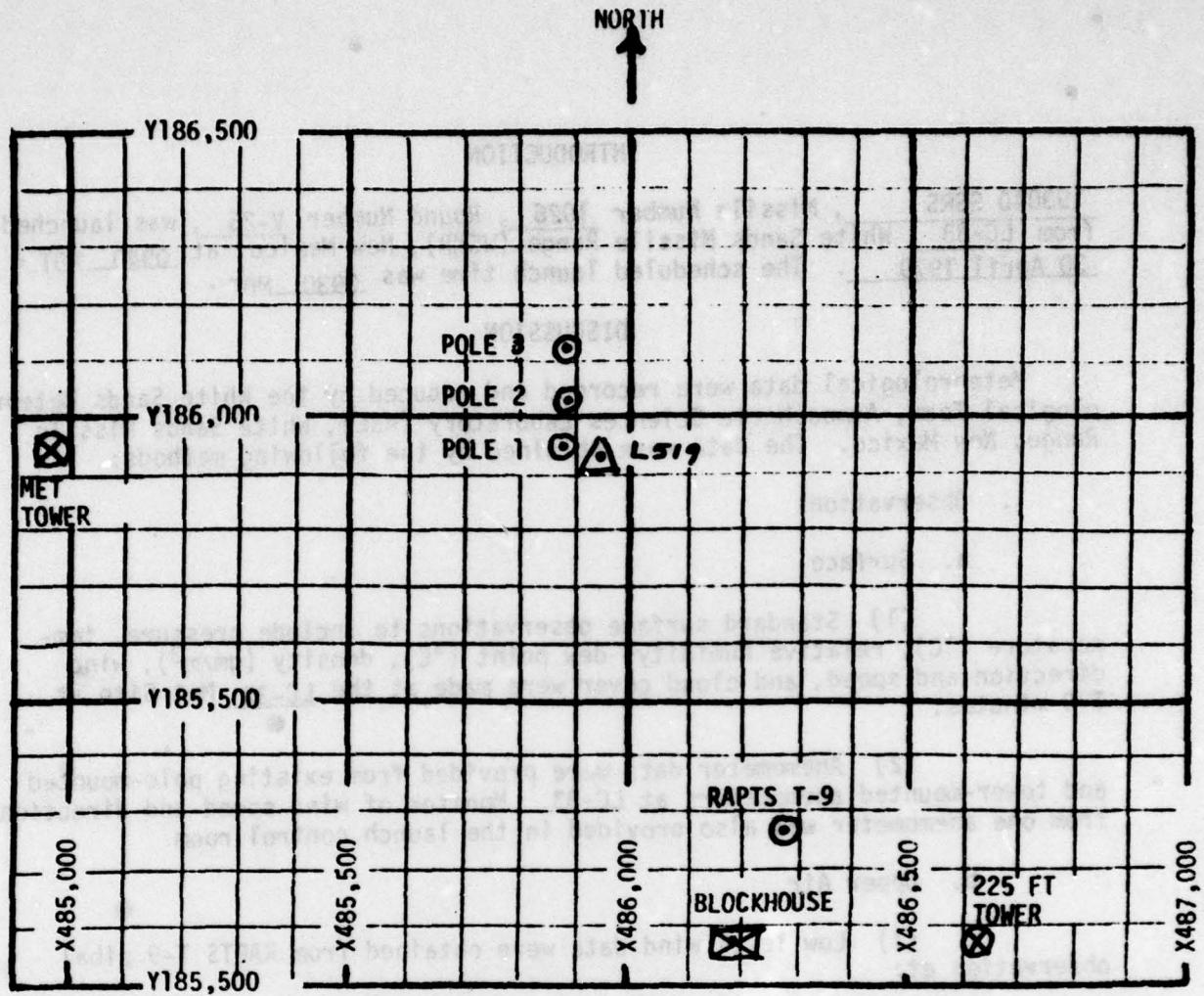
1. MET TOWER - 4 Bendix Model T-120 Anemometers at 12 ft, 62 ft, 102 ft and 202 ft with E/A recorders.
