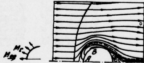
(d) injection with M_c = 0.5 , distributed over surface A to B.
