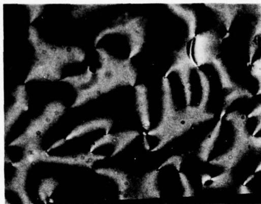
Fig. IV-5. An optical micrograph is shown of a 50- \mu\text{m} -thick slab of MBBA in the nematic phase confined between smooth amorphous substrates. The slab is observed between crossed polarizers. Several wedge disclinations are visible.
