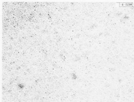
Fig. V-19. Transmission electron micrograph of gold islands on an amorphous \text{SiO}_2 surface with a 1.5-nm-deep, 320-nm-period, square-wave surface-relief grating fabricated using ion-beam etching. The magnification is \approx 100 \text{ KX} .
