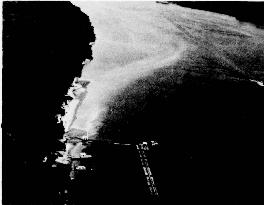
Figure 7. Turbidity from pipeline dredge disposal operations
