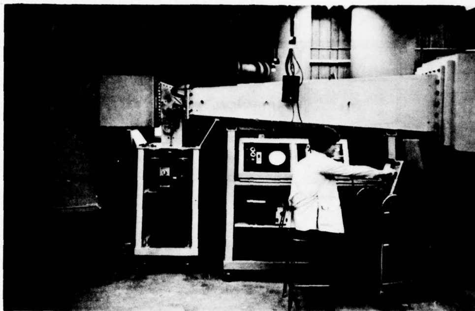
FIG. 11. VIEW OF THE SMALL END OF THE HORN SHOWING ALSO THE LARGE TANK OF THE AIR RESERVOIR SYSTEM, FLAP VALVE AND ELECTRIC-MOTOR DRIVE SYSTEM, CONTROL CONSOLE, AND ANCILLIARY ELECTRONICS.
