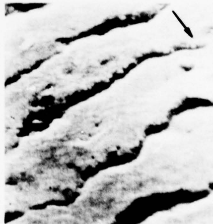
Plate 38 10 μ S.E.M. of Ti-alloy (IMI 318) 200°C, 247 ± 139 MN/m 2 210 000 cycles
