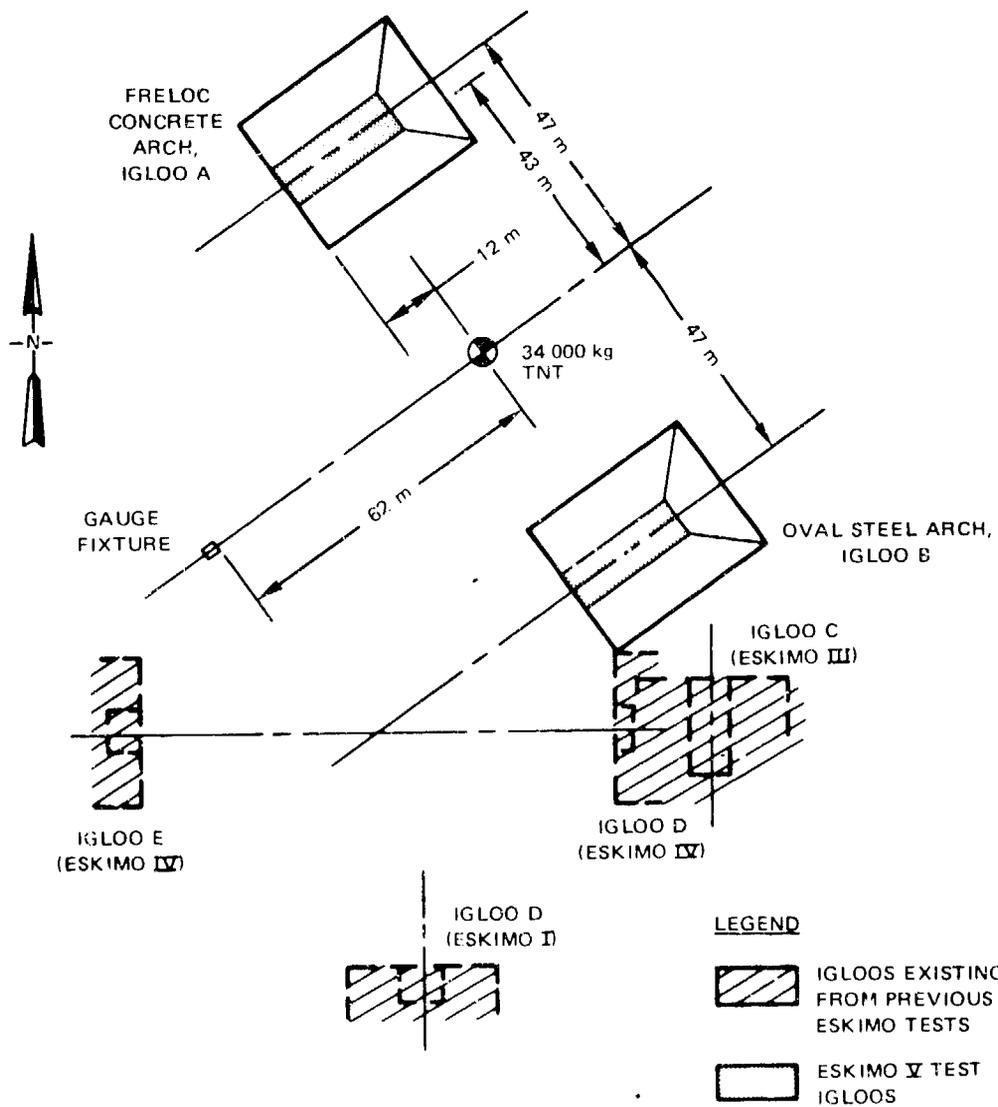
FIGURE 2. ESKIMO V Test Area Layout.
