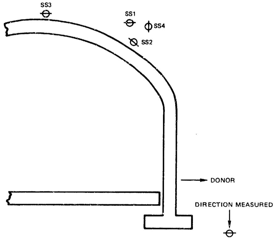
FIGURE 15 Soil Stress Gauge Locations, FRELOC Igloo.
