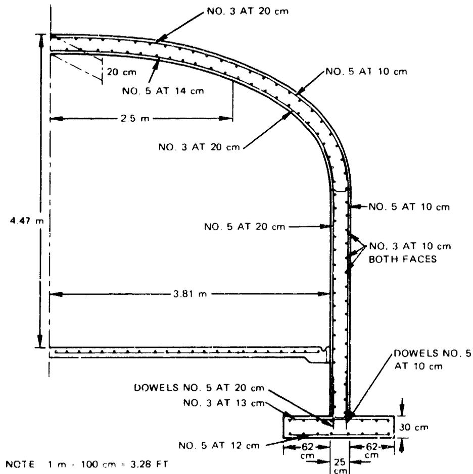
FIGURE 4. Half-Section of FRELCO Igloo Test Structure.
