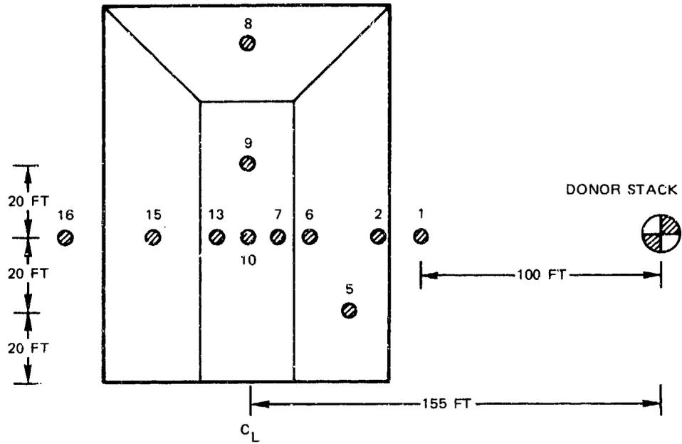
FIGURE 13. Electronic Blast Gauge Layout on FRELOC Igloo.
