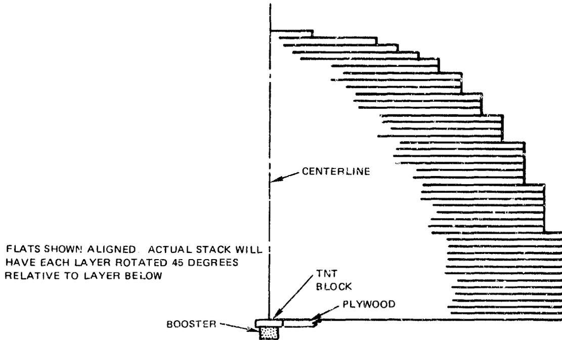
FIGURE 11. Vertical Section of One-Half TNT Donor Stack.
