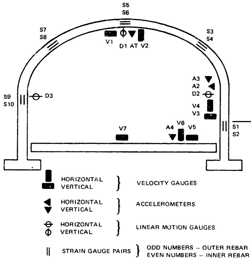
ADDITIONAL GAUGE PAIRS S11,S12, AND S13,S14 CORRESPONDING TO S5,S6 WERE LOCATED 20 FT AND 2 FT RESPECTIVELY FROM THE HEADWALL
