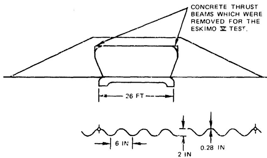
FIGURE 8. Cross Section of Oval Steel-Arch Magazine.
