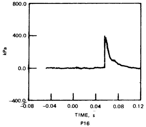
FIGURE 42. Overpressure Gauges P7, P13, P15, and P16, Igloo A.
