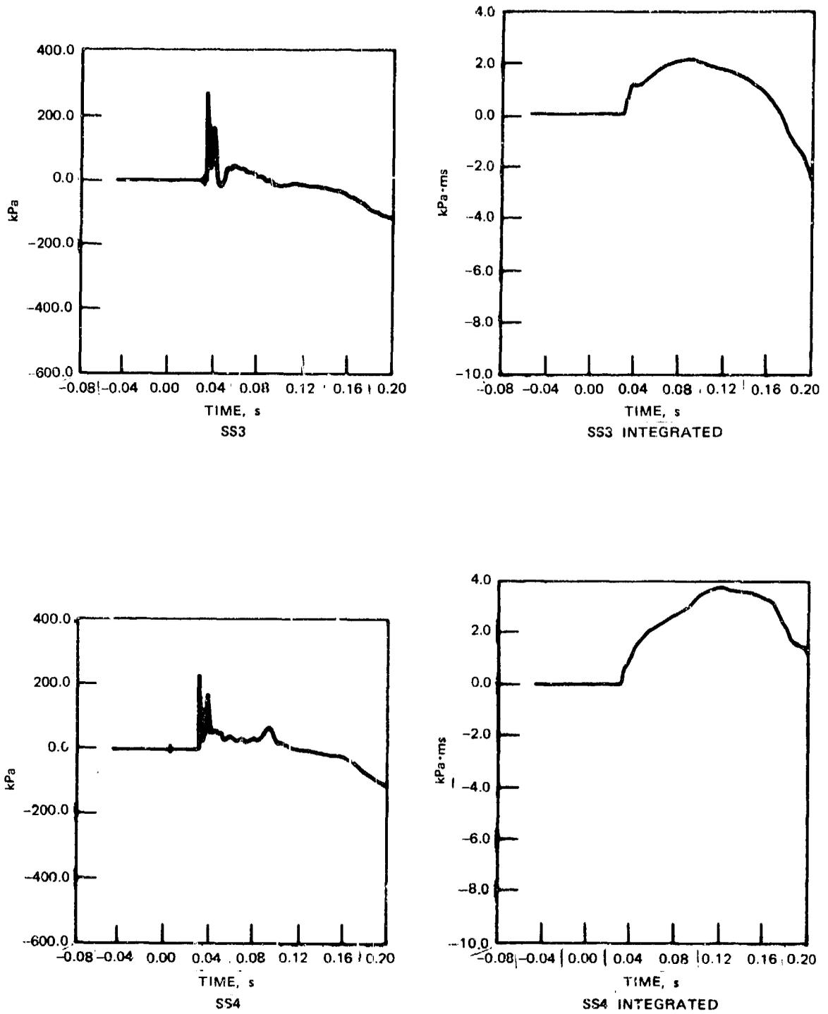
FIGURE 50. Data Plot: for Soil-Stress Gauges SS3 and SS4.
