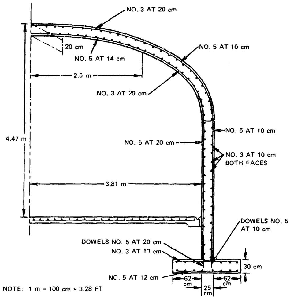
FIGURE A-1. Half-Section of Test Structure.
