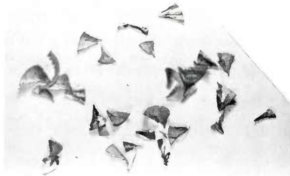
Fig. 16: Chips Produced in High Density P/M Materials a) f = 0.003 ipr; b) f = 0.005 ipr; c) f = 0.009 ipr
