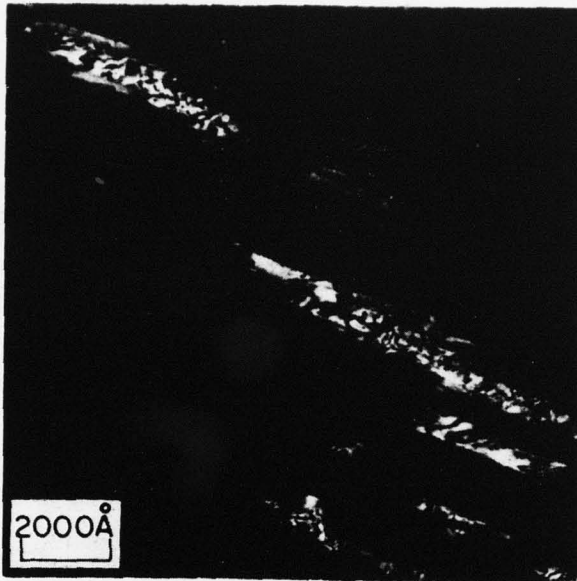
Fig. 4 - Dark field electron micrograph showing monolithic laths of type 1 \alpha in a Ti-12wt%Mo-6wt%Al alloy.
