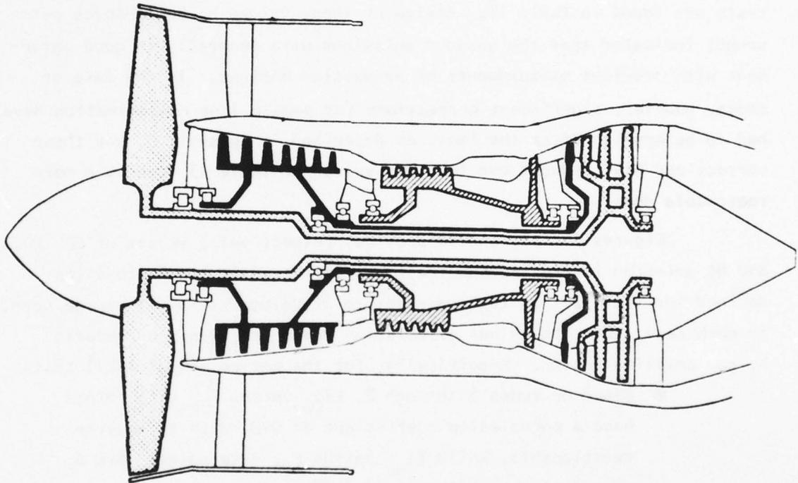
Figure 33. RB211-22B Schematic
