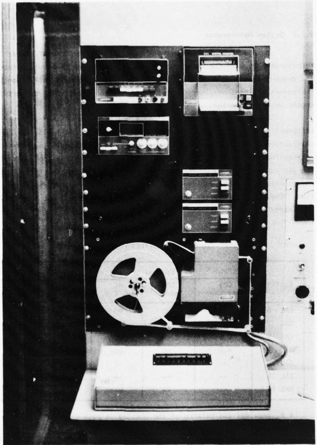
Figure 8. Digital Recording System
