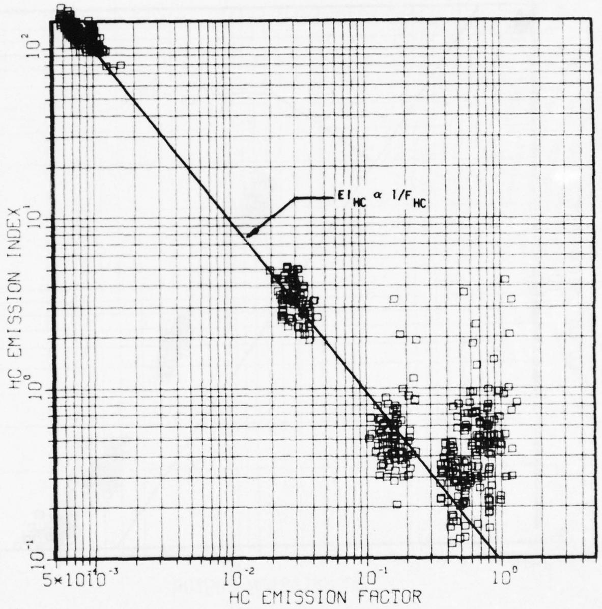
Figure 25. JT3D-3B Uncorrected HC Emission Data
