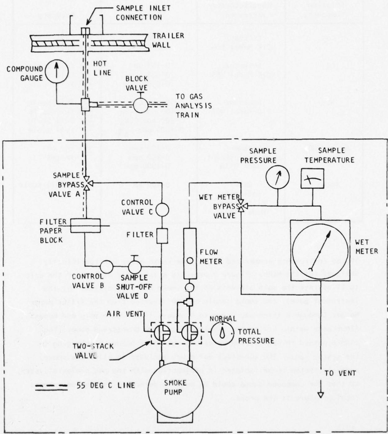
Figure 7. Schematic Diagram of NREC Model 1974 Smoke Meter
