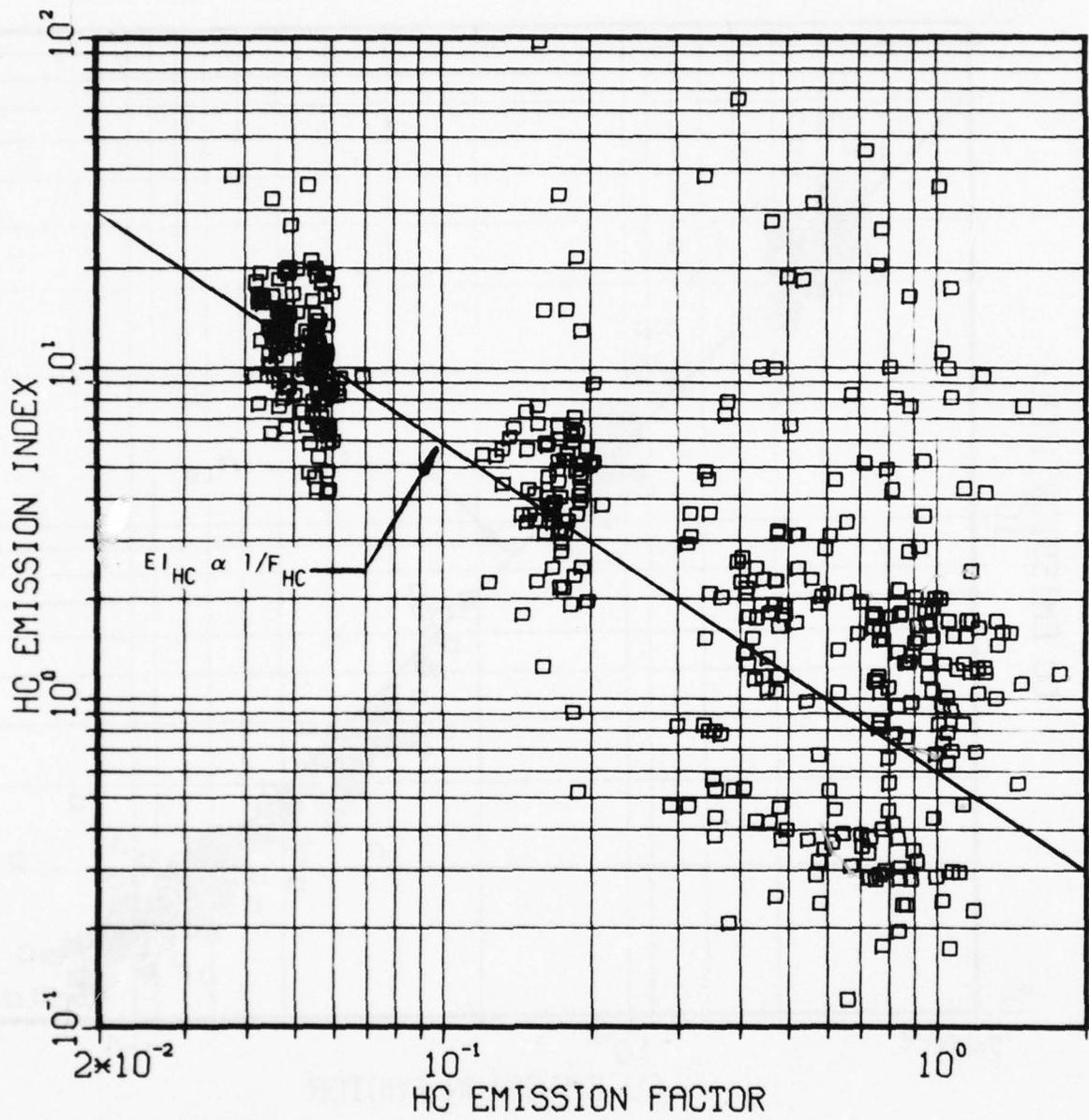
Figure 12. JT8D-9 Uncorrected HC Emission Data
