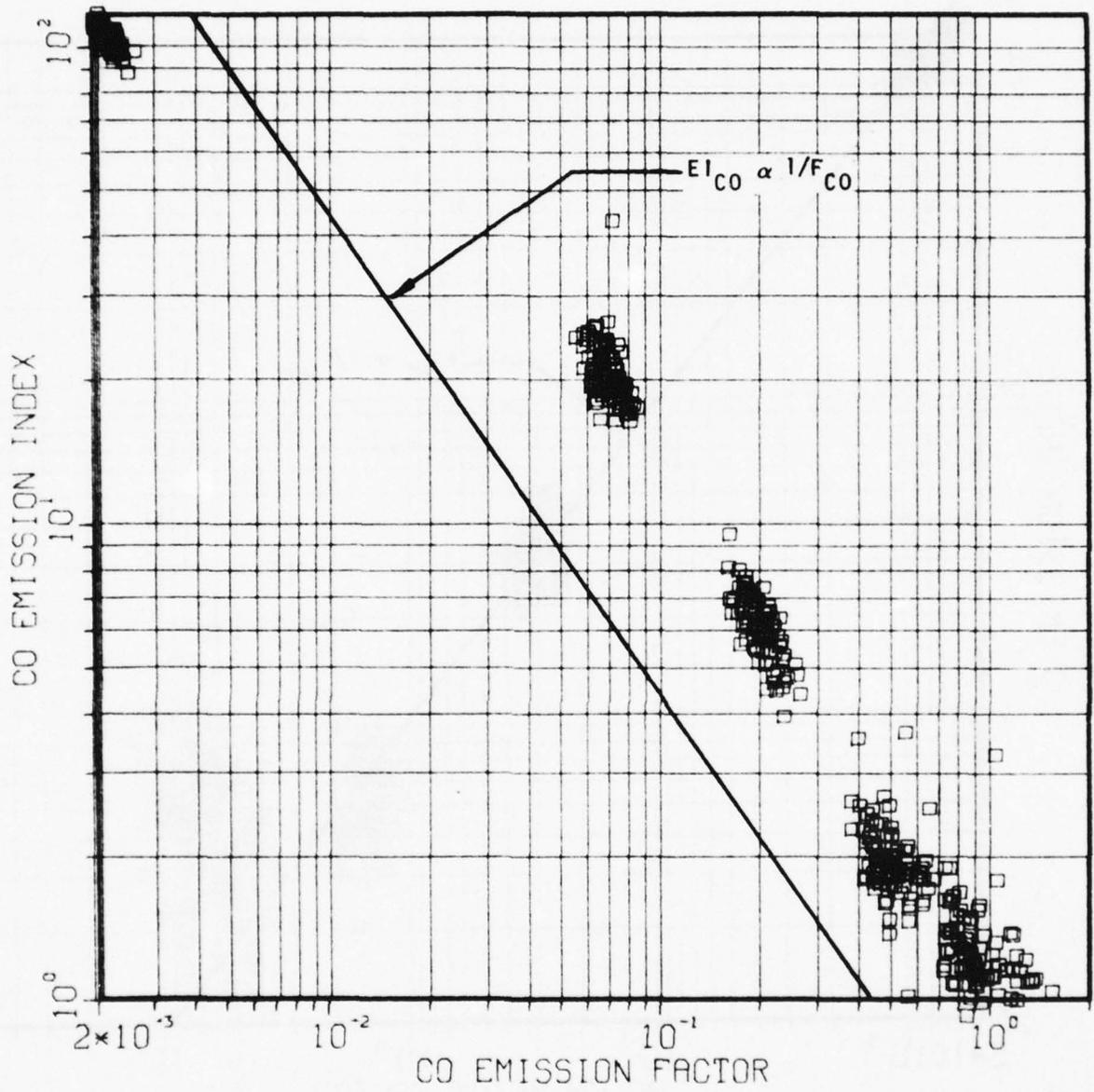
Figure 24. JT3D-3B Uncorrected CO Emission Data
