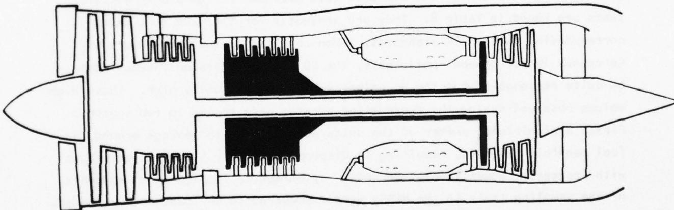
Figure 10. JT8D-9 Schematic
