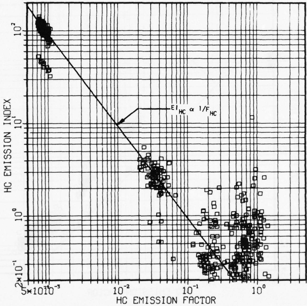
Figure 20. JT3D-7 Uncorrected HC Emission Data
