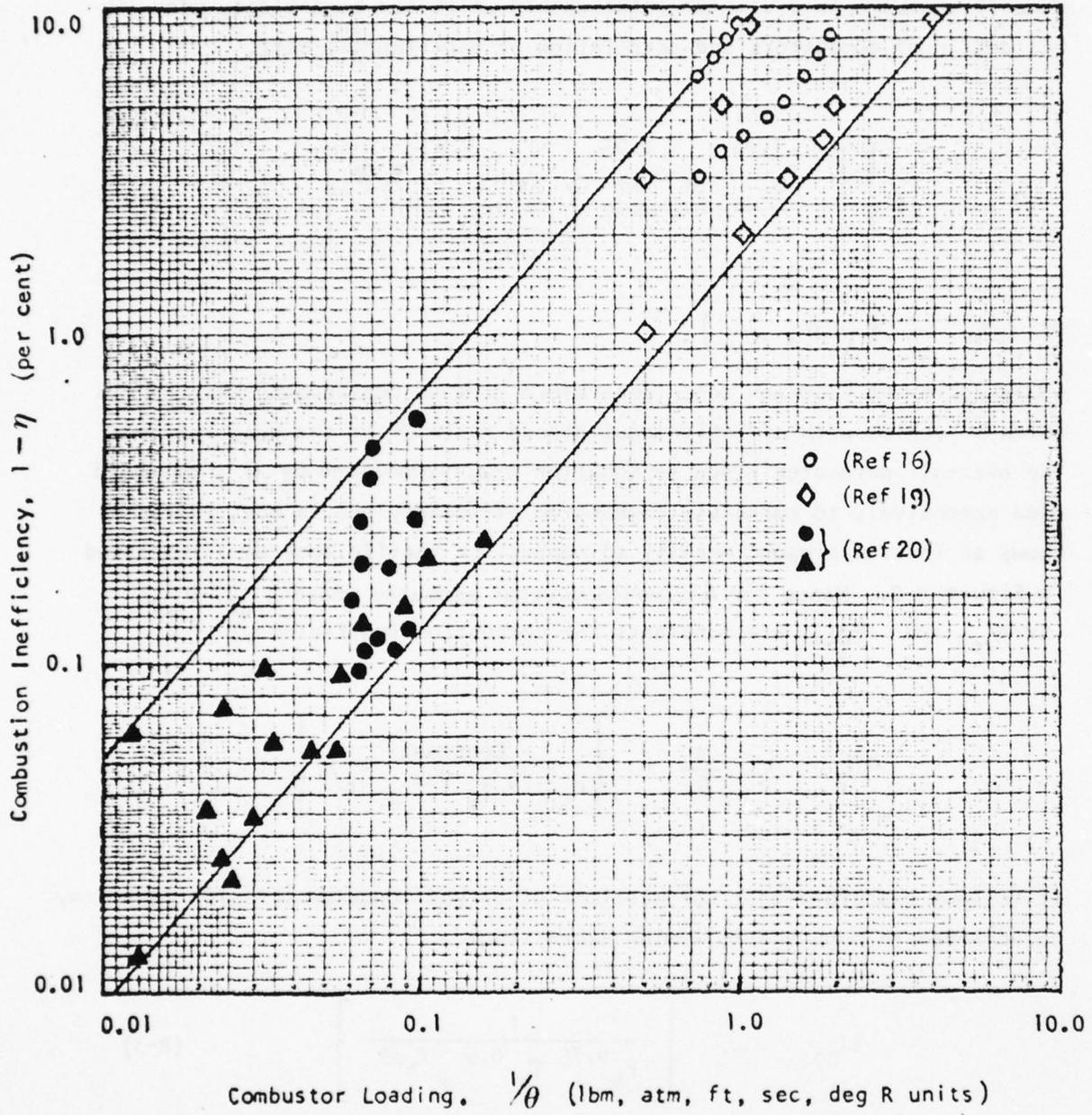
Figure B-2. Combustion Inefficiency Correlation
