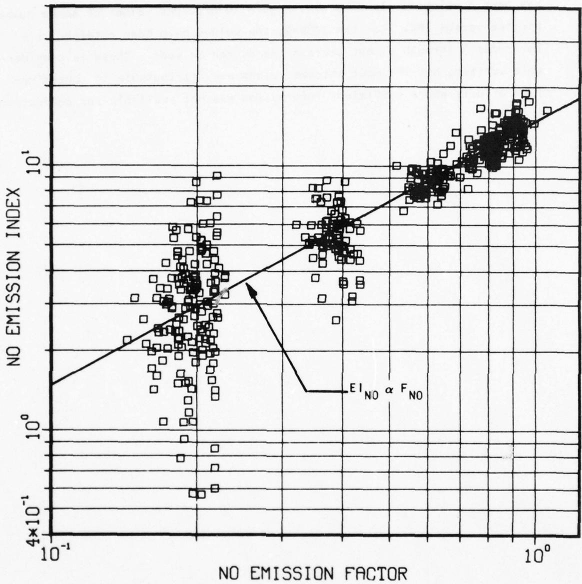
Figure 13. JT80-9 Uncorrected NO Emission Data
