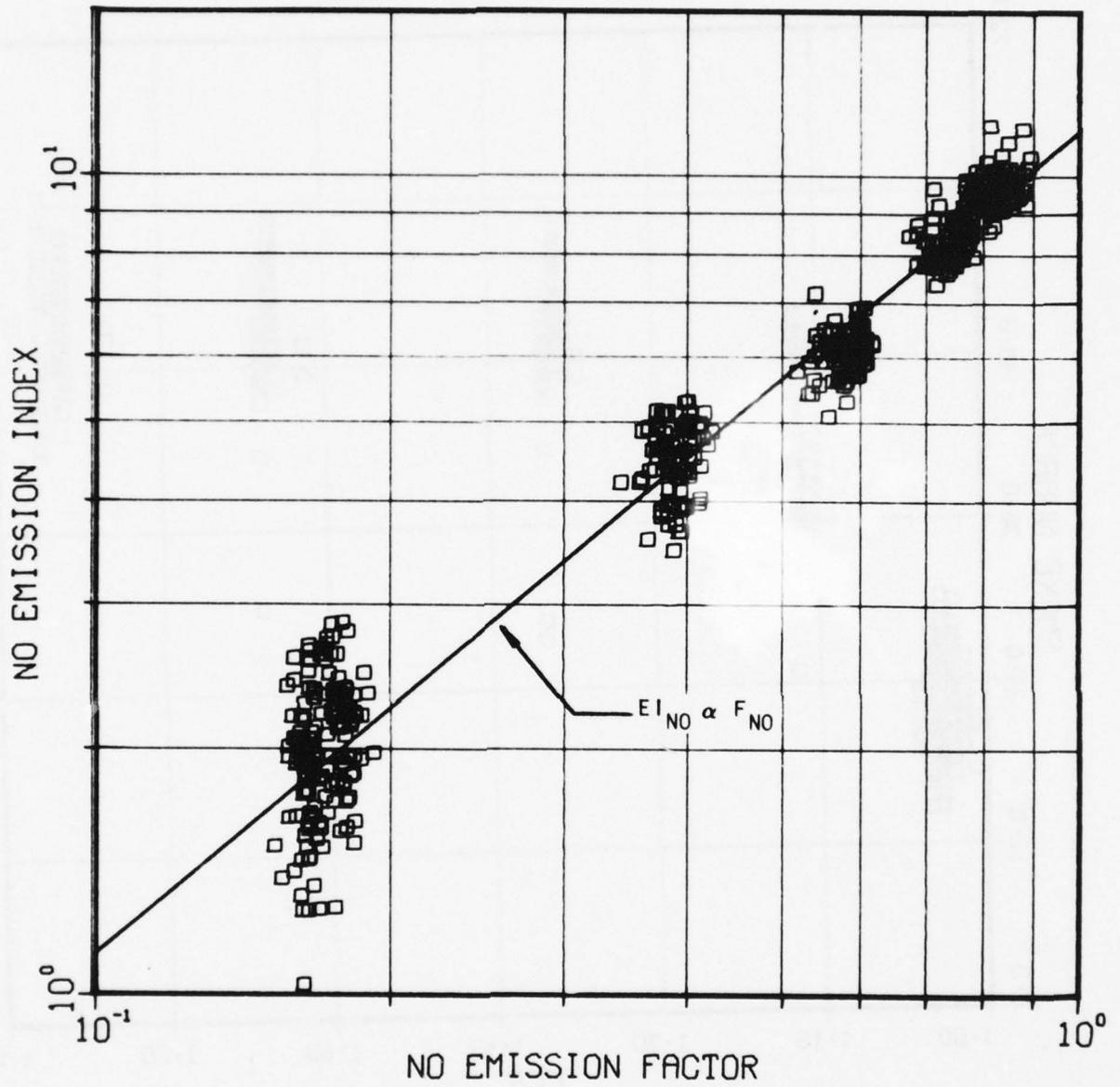
Figure 26. JT3D-3B Uncorrected NO Emission Data
