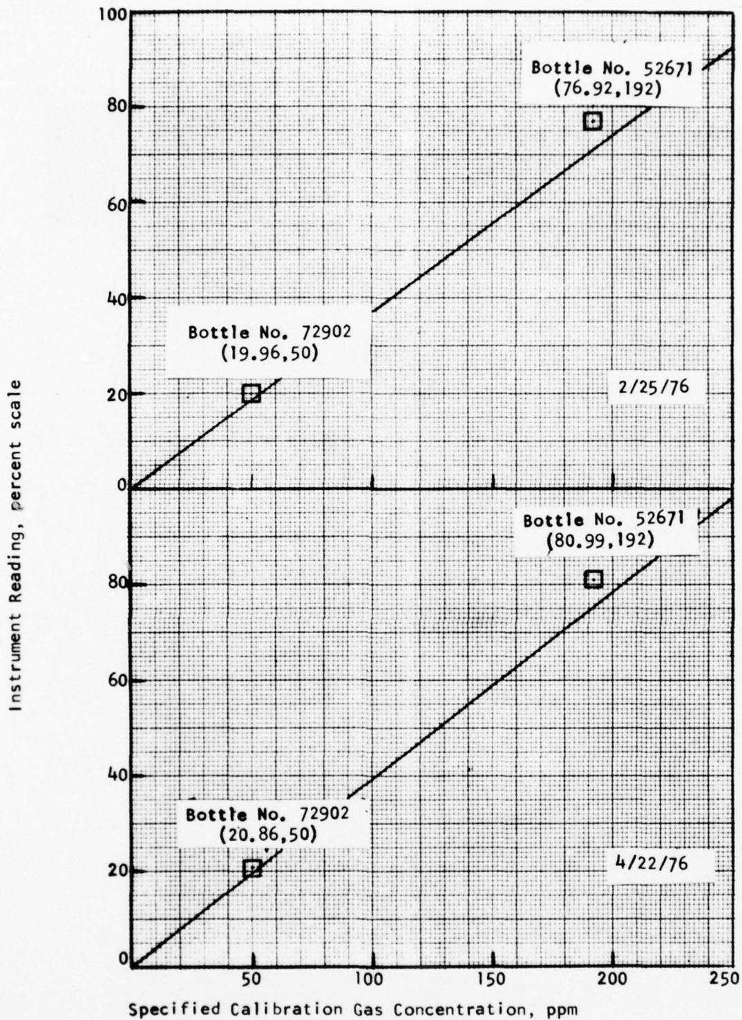
Figure D-2. Monthly NO Calibration - Range 2
