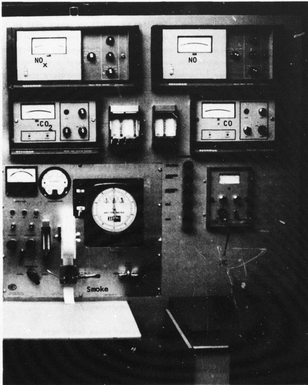
Figure 6. Mounted Gas Analyzers and Smoke Meter
