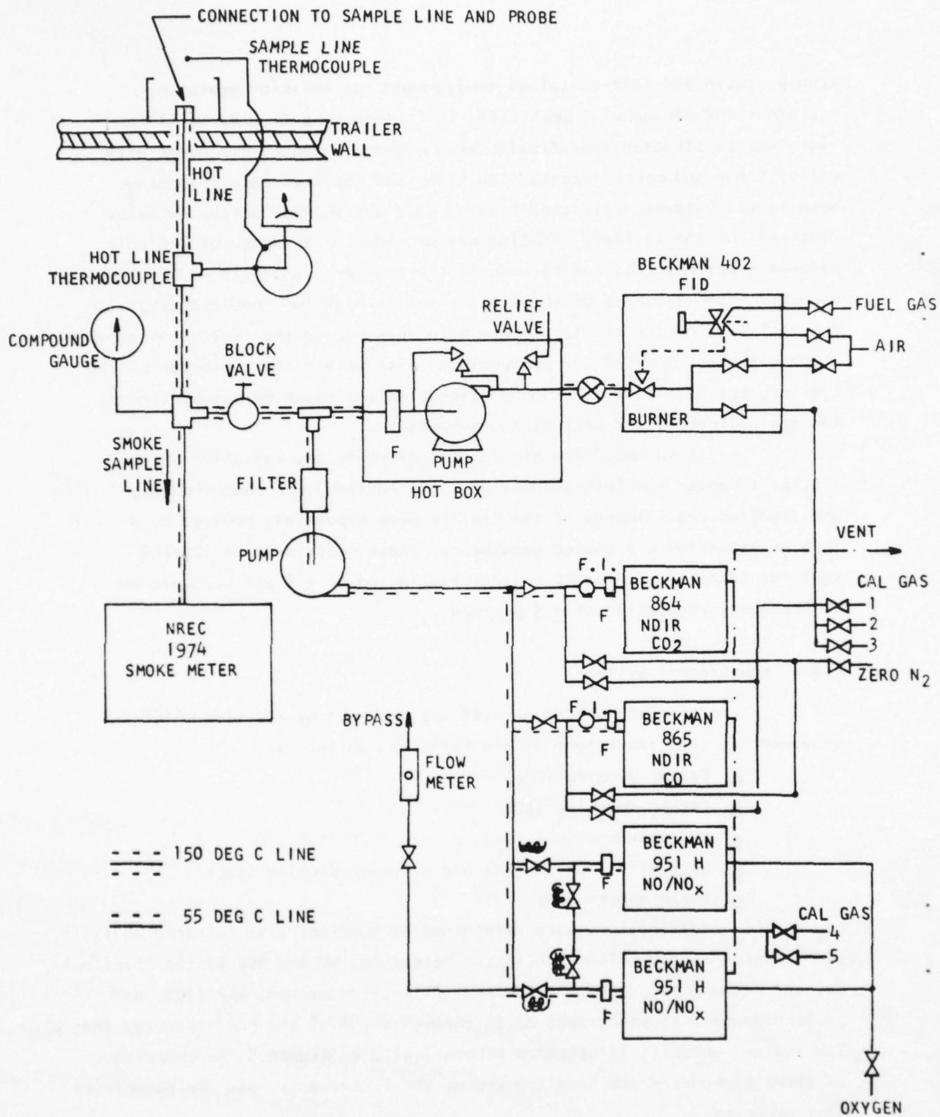
Figure 5. Measurement System
