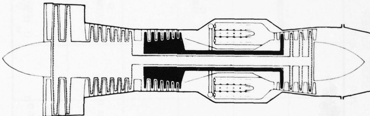
Figure 23. JT3D-3B Schematic
