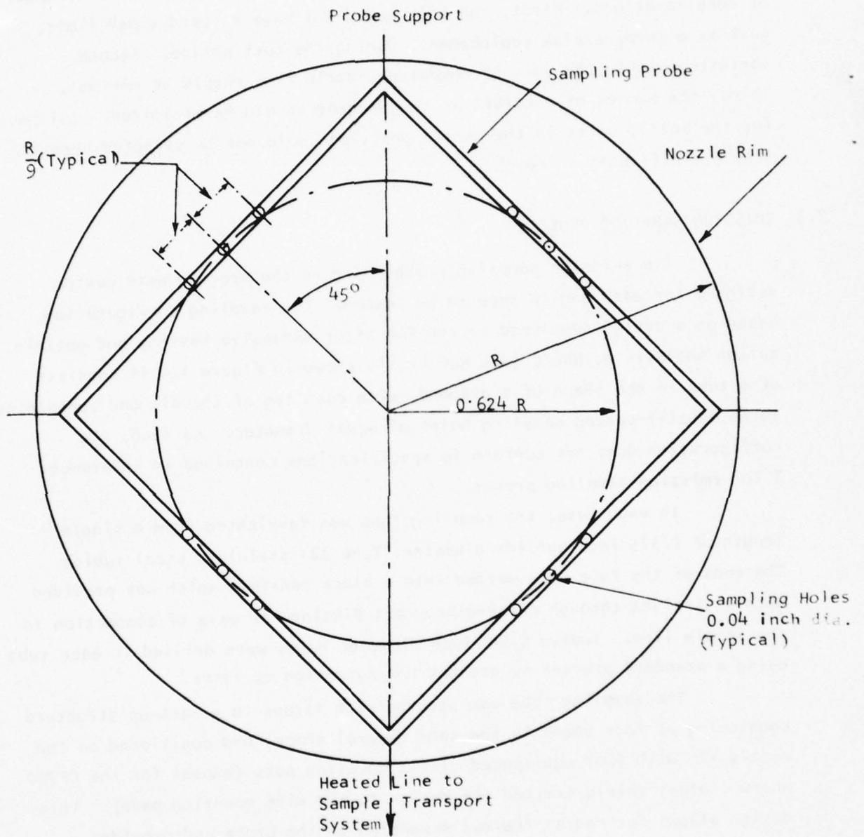
Figure 1. Sampling Probe Configuration
