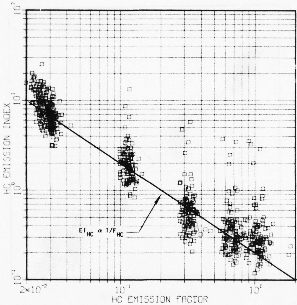
Figure 16. JT8D-7 Uncorrected HC Emission Data
