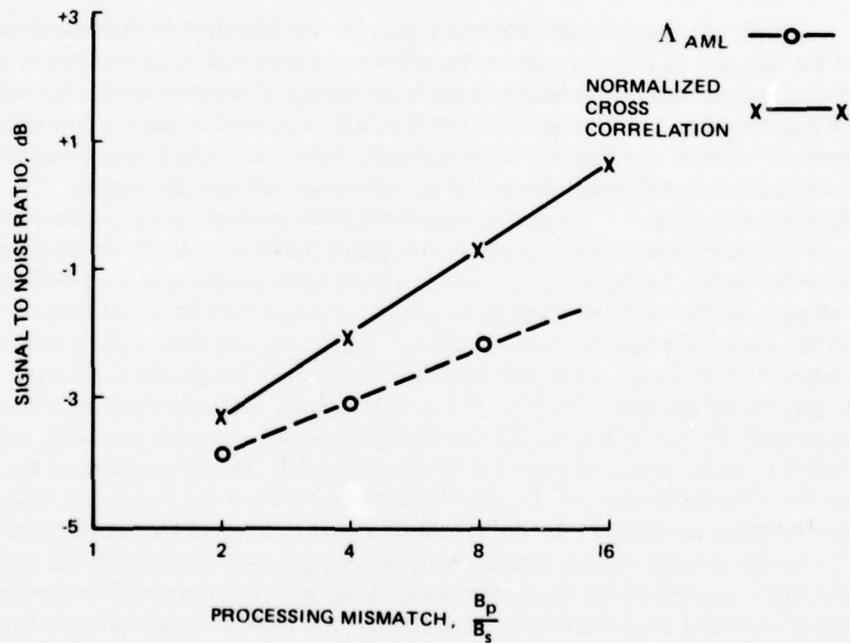
Figure 5. Signal to noise ratio necessary to obtain a probability of detection of 0.5 as a function of the mismatch of processing bandpass to signal bandpass;  $P_{FA} = 10^{-3}$ .
