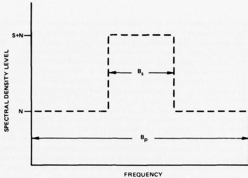
Figure 4. Depiction of processing mismatch to the signal bandwidth. Signal possesses a bandwidth of  $B_s$  and a spectral density of  $S$ . Processing bandpass is  $B_p$  with a noise spectral density of  $N$ .
