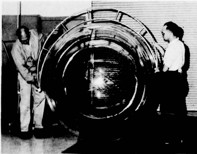
Figure A.23. Measuring the external diameter at selected locations.
