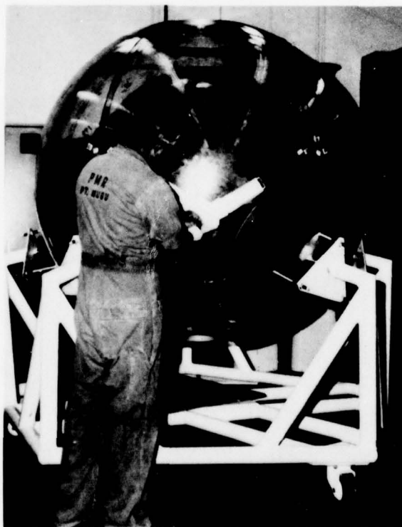
Figure A.18. Aligning two hemispheres prior to bonding of the equatorial joint.
