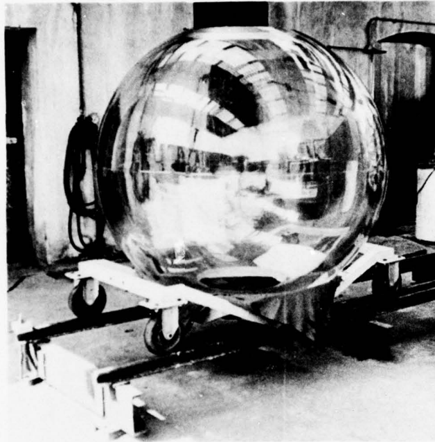
Figure A.45. Bonded sphere after sanding, polishing, and annealing.
