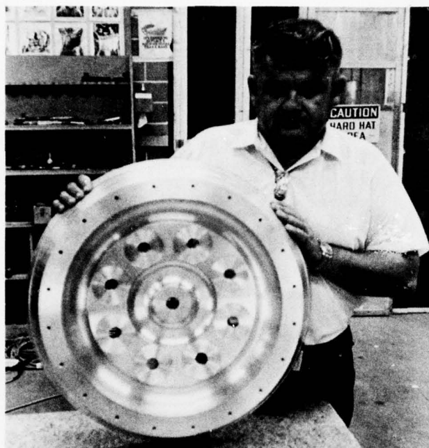
Figure A.49. Aluminum penetration closure serving as a bulkhead for feedthroughs.
