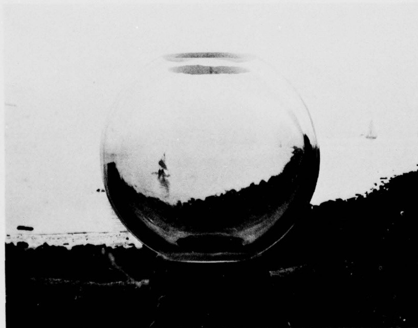
Figure A.48. Completed sphere prior to installation of penetration closures. Note that the equatorial joint is almost invisible.
