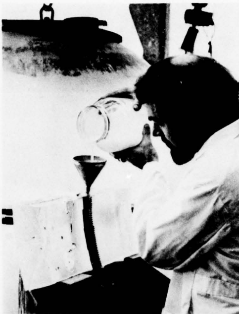
Figure A.43. The joint in a bond test specimen is filled with the same casting slurry as the equatorial joint in the sphere.
