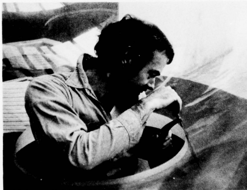
Figure A.46. Measuring the thickness of the casting at the penetration.
