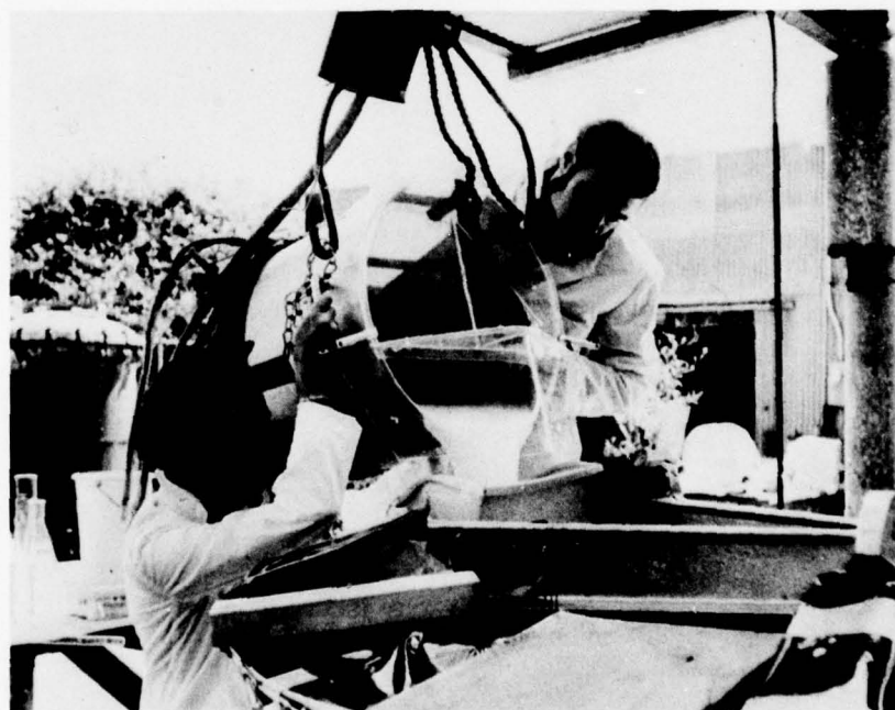
Figure A.32. Pouring degassed casting slurry into the annular space between the male and female molds.
