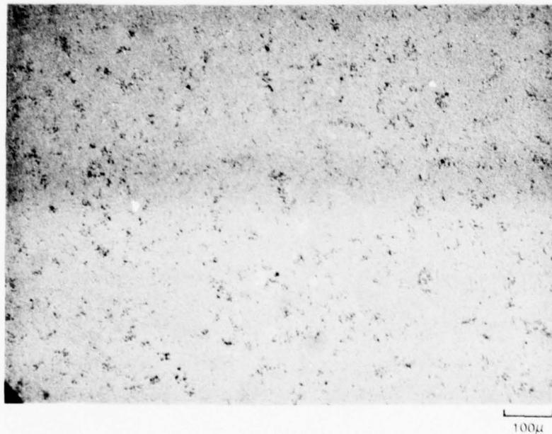
Fig 35. Polished and HF Etched Surfaces of ( $\beta'$ -X) Sample 27.3.3
