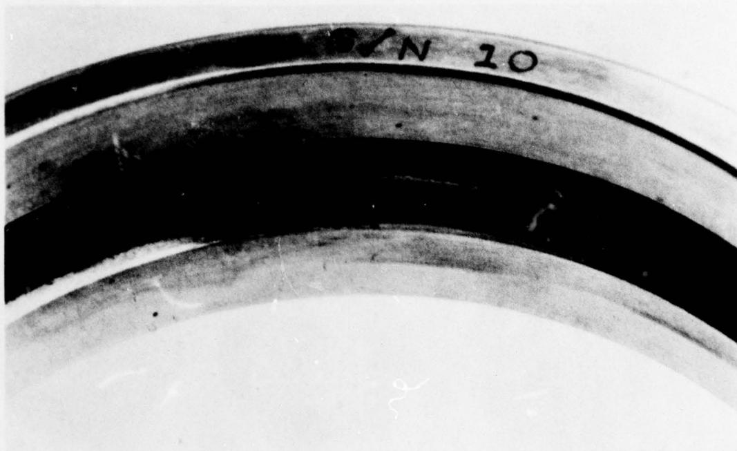
*Figure 18. Outer Race of Silicon Nitride Bearing After Oil Shutoff Test*
