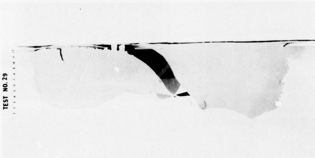
Figure 16. Combined Fragment and Blast Damage to Thinner 7075-T6 Aluminum Front Panel Tested with Empty Fuel Tank
