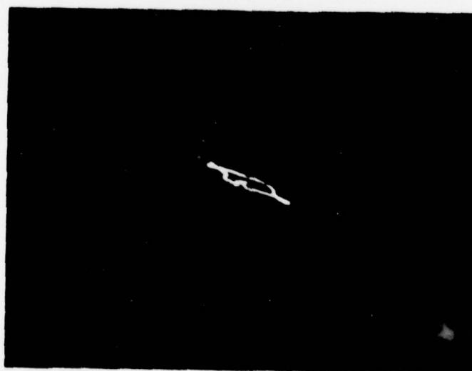
PHD-0618-2-79 Figure 15. Eddy Current Indication Caused by .020" Deep Notch in Test Standard
