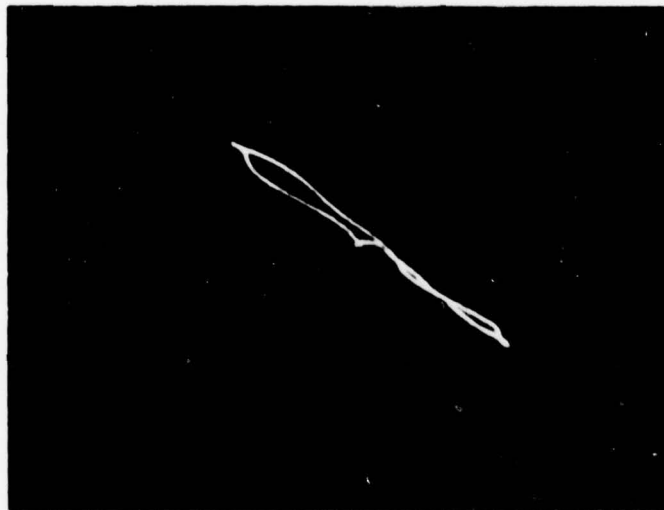
PHD-0619-2+79 Figure 16. Eddy Current Indication Caused by Naturally Occuring Flaw
