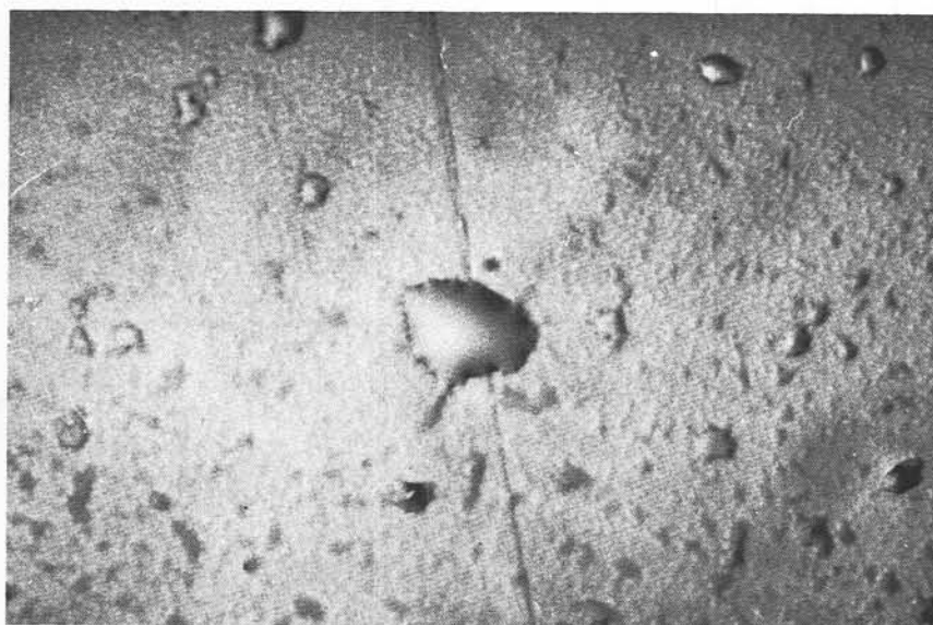
Figure 11. Gas bubbles produced on K.D.P. by electron bombardment
