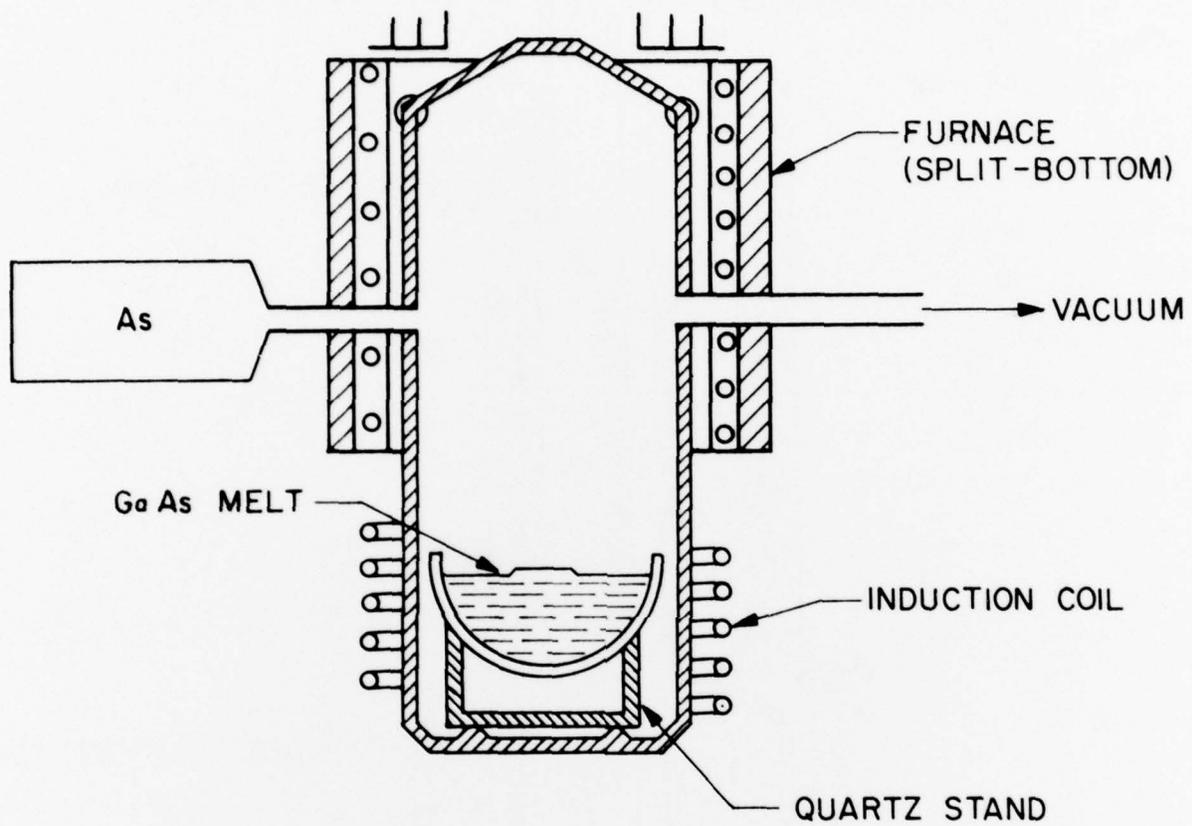
FIGURE 2. GaAs GROWER WITH NO PULLING APPARATUS
