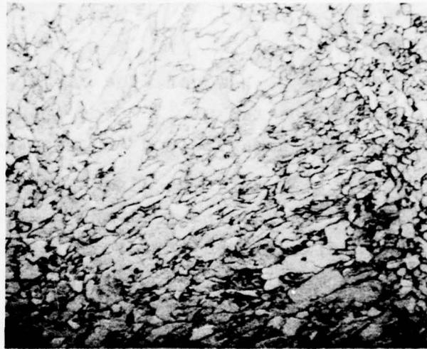
a. 0.010 in. (0.25 mm) Thick Layer. Layer Removed in Decementing Agent prior to Etching.
