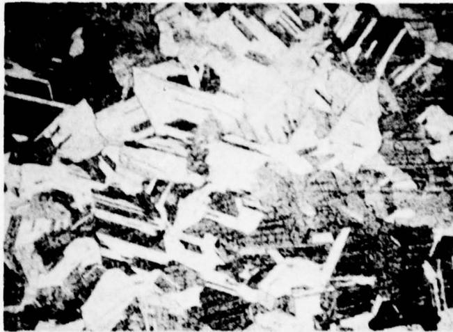
a. Standard Grain Size, Thin Specimen
