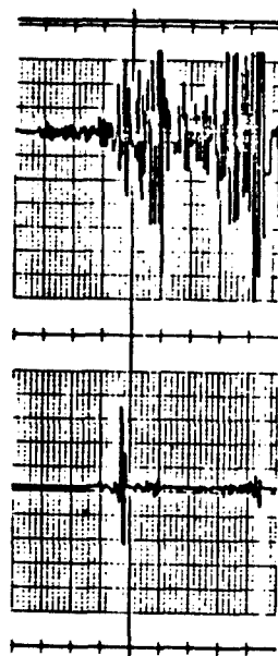
0.070" LONG CRACK (NATURAL FLAW)
