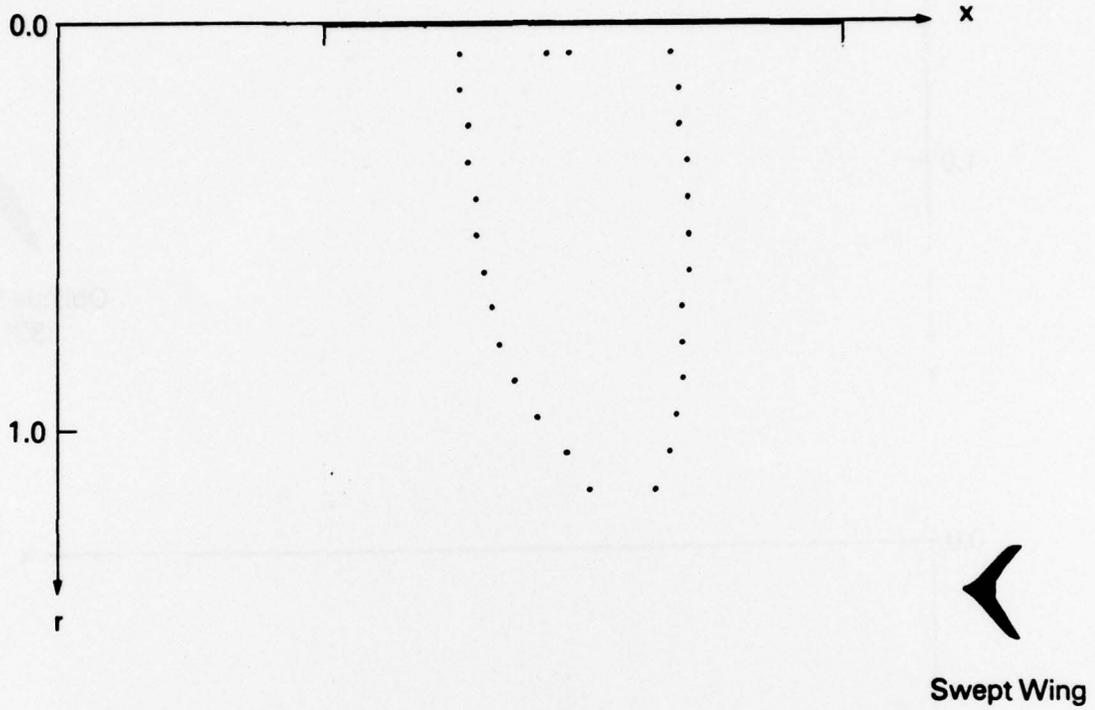
Figure 6-b. Sonic Lines of Axisymmetric Flows Around Equivalent Bodies (Cont.).
