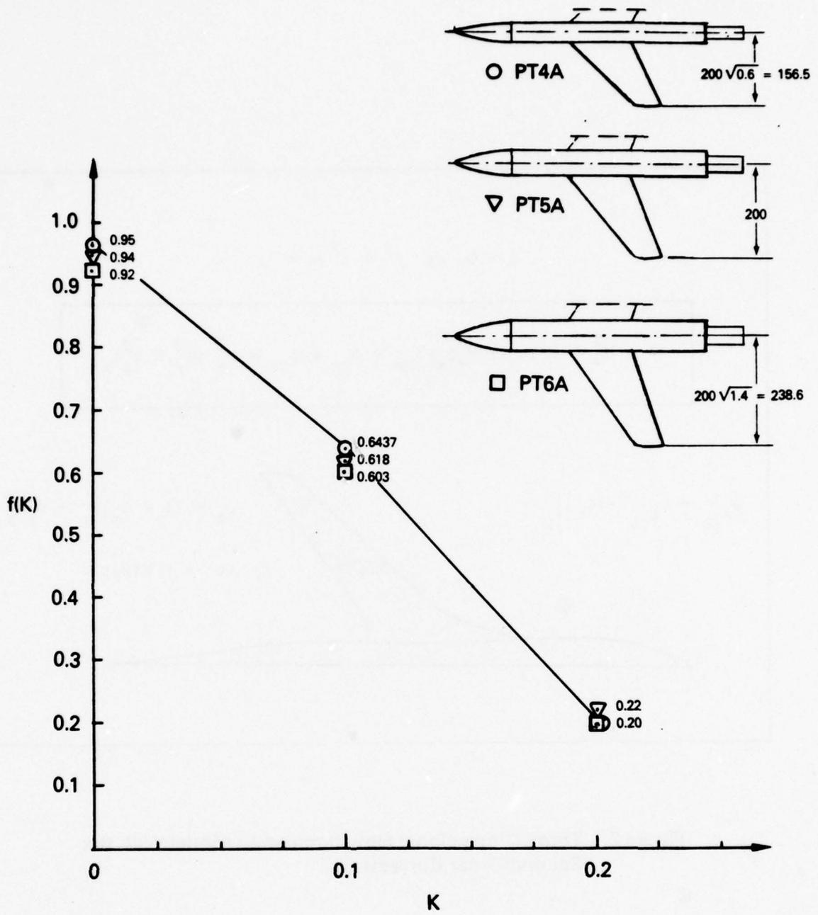
Figure 3. Drag Rise Correlations According to Transonic Equivalence Rule Formulation Based on FFA Experimental Data.
