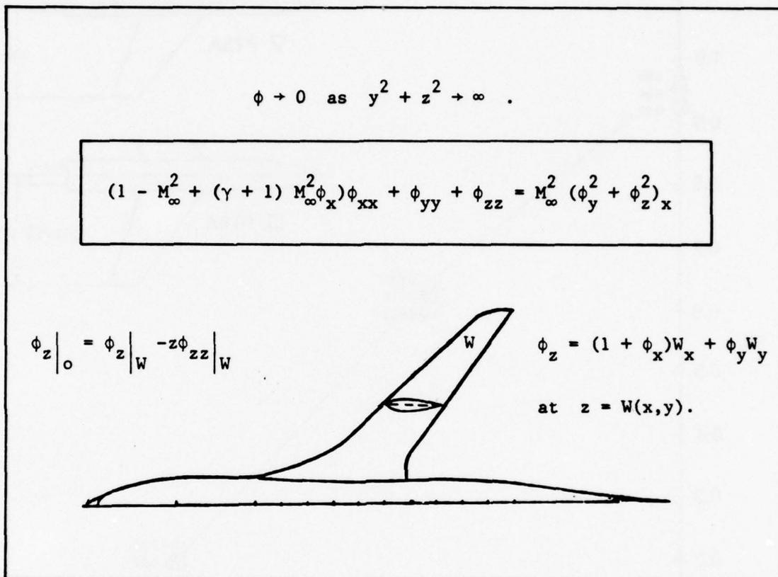
**Figure 2. Three-Dimensional Flow Simulation Model With the Second Order Corrections.**
