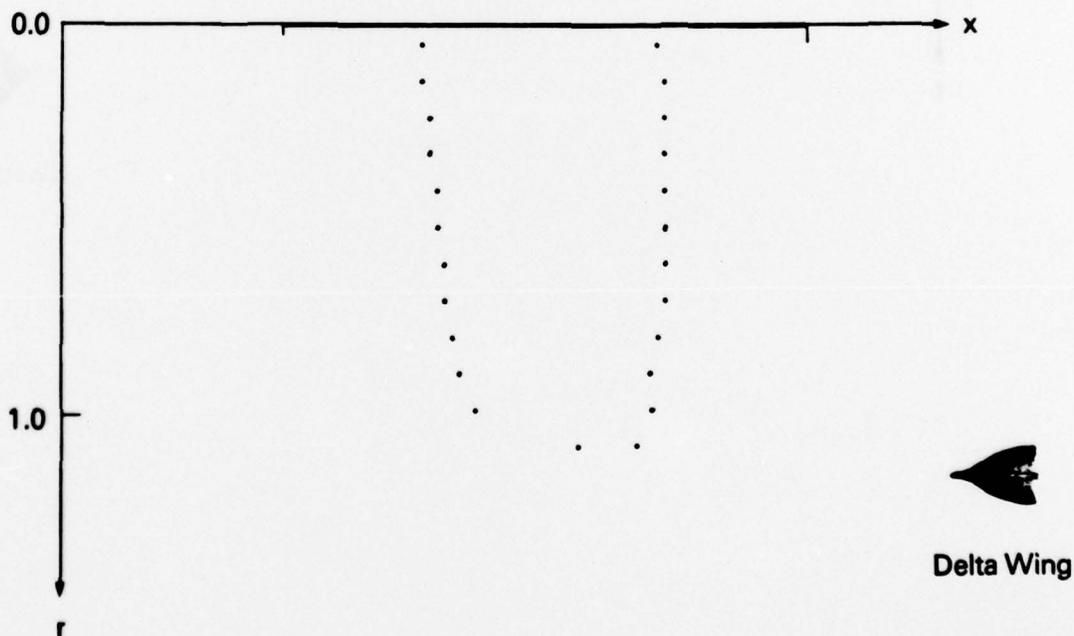
Figure 6-b. Sonic Lines of Axisymmetric Flows Around Equivalent Bodies (Cont.).
