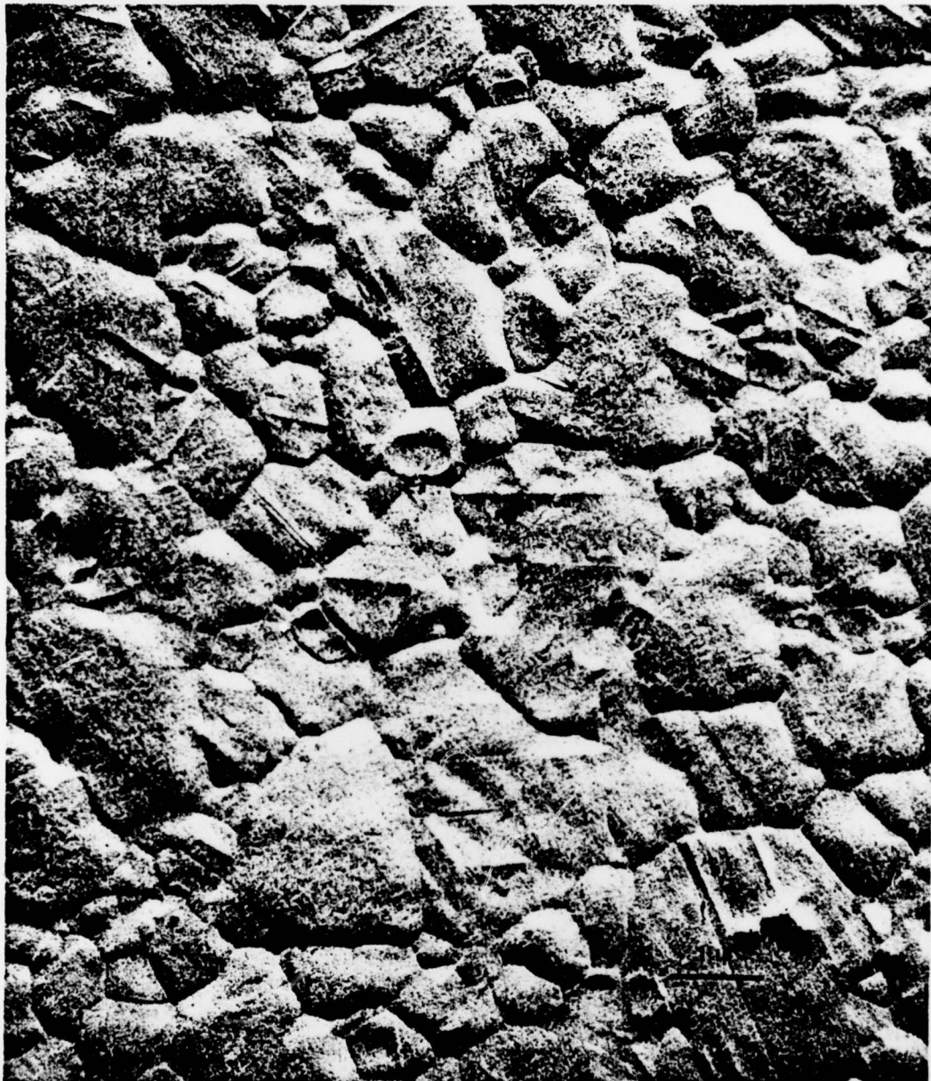
Figure 6. Carbon replica of a typical sputter etched film; note the wide grain size distribution.
