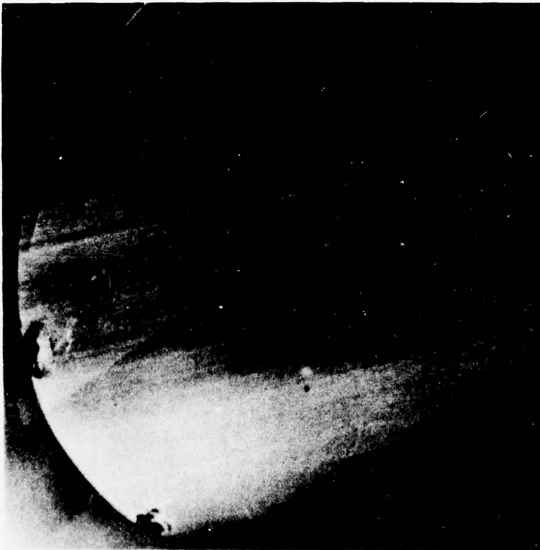
Figure 3-12. X-ray Topograph of a Wafer from HgCdTe Ingot WK-9
